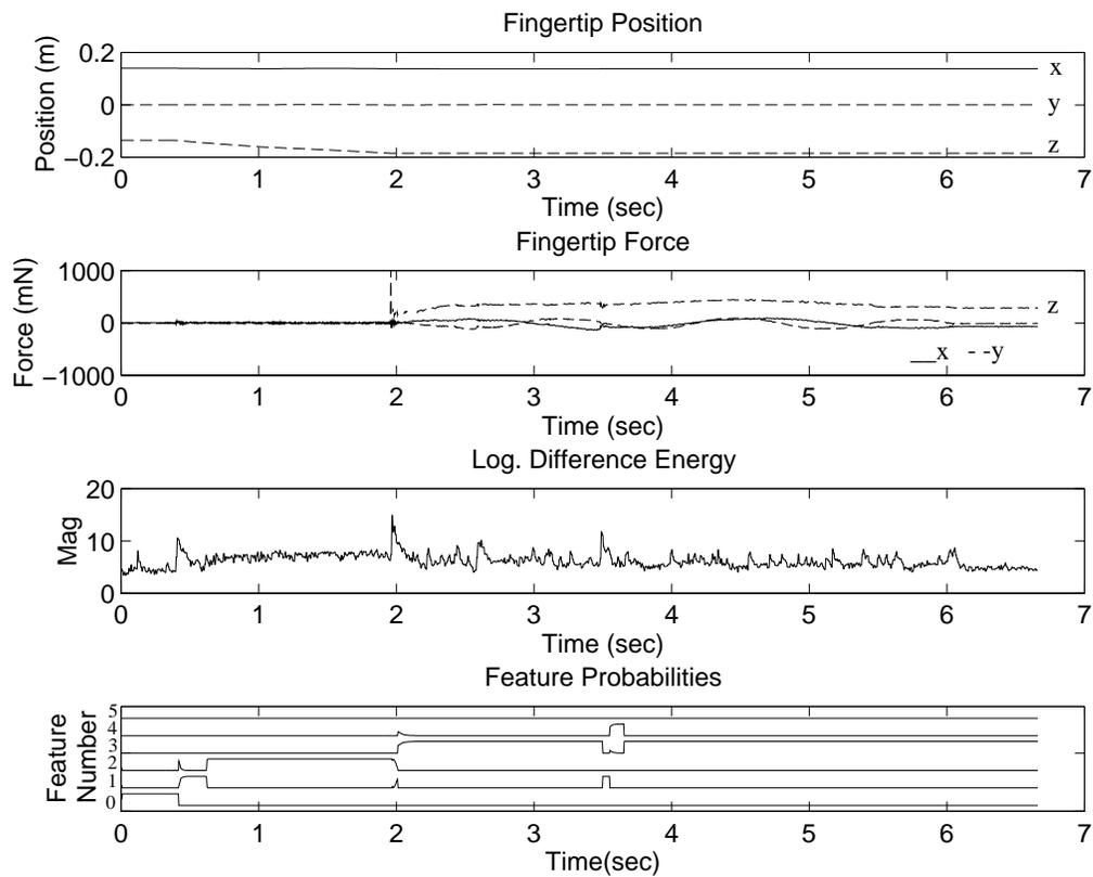
Figure 9.1: Example simple guarded move trace. The top plot shows the position of the fingertip. The  $x$ ,  $y$ , and  $z$  plots are labeled in the figure. The next plot shows the force on the fingertip with the same line-type convention. The next plot shows the logarithm of the strain difference energy. The bottom plot shows the probability traces for each feature.
