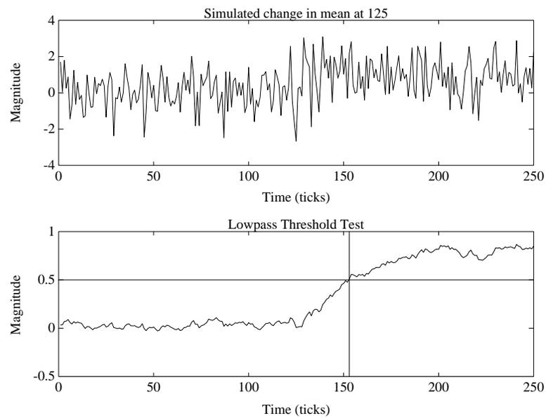
Figure 6.6: Lowpass filter of  $x(n + 1) = 0.98x(n) + 0.02y(n + 1)$  on the same signal as figure 6-3. The threshold is 0.50. The change is detected at 153. This is a slower response than the response for the PH test. Further, an estimate of the change time is not computed.
