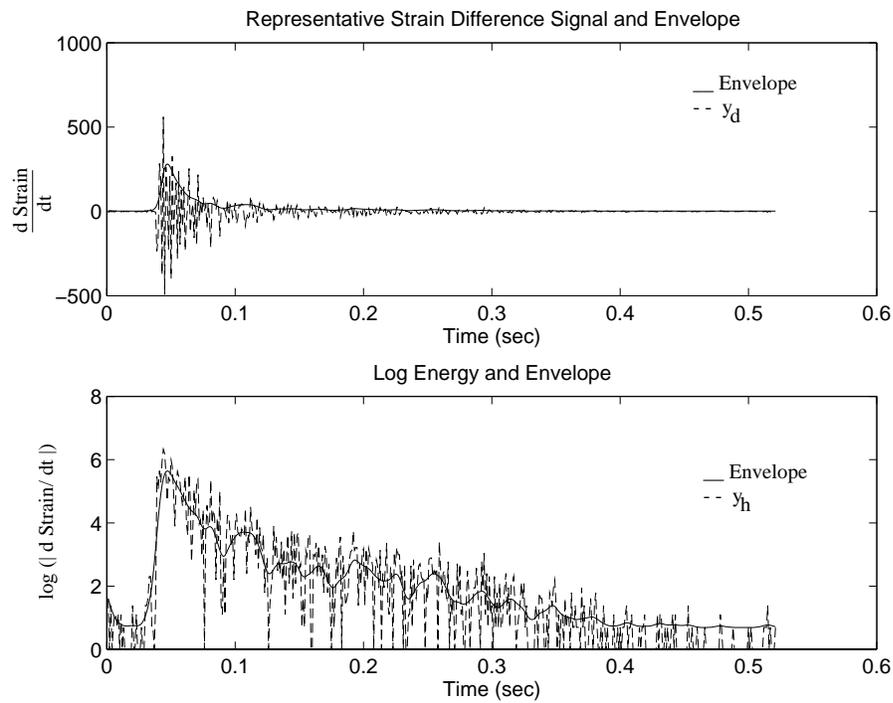
Figure 7.3: Characteristics of an impact process. The primary characteristic is the sharp rise in strain followed by vibration within an exponentially decaying envelope. The upper figure shows the difference signal and an exponential envelope fit from the logarithmic trace. The lower figure shows the logarithm of the absolute value of the difference signal and an envelope created by lowpass filtering.
