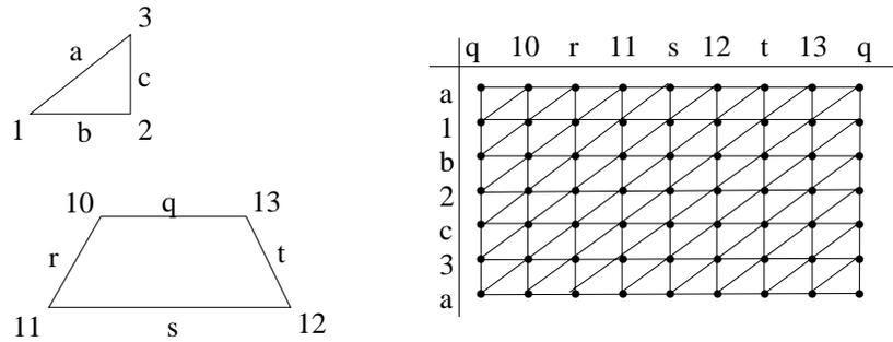
Figure 4.4: Path connectivity of the configuration space topology for the indicated convex objects. The configuration space is the  $(x, y, \theta)$  coordinates of the triangle. Each dot in the matrix indicates a possible pairing between features on the triangle and features on the parallelogram. A segment indicates the pairings are connected. The other diagonal direction does not appear because those segments represent paths that cause objects to pass through each other.
