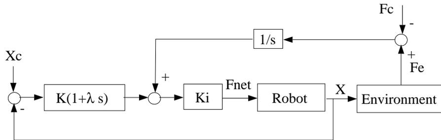
Figure 9.3: Integral endpoint force controller with position feedback.
