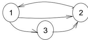
where 3 is the transient feature node. In this model, the impact node can only be visited when transitioning from free space to contact. In some cases, there may be sufficient stored energy in the sensor so that a release impact occurs when transitioning from contact back to free space.
