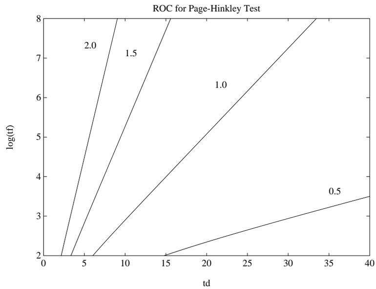
Figure 6.3: Receiver operating characteristic (ROC) of Page-Hinkley test between two Gaussian distributions with different means and the same variance as a function of the signal to noise ratio  $s = \frac{\Delta\mu}{\sigma}$ . The  $\log_{10}(\bar{t}_f)$  is shown as a function of the mean time to detection  $\bar{t}_d$  for  $s = 0.5, 1.0, 1.5,$  and  $2.0$ .
