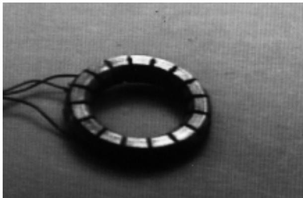
**Figure 7-1:** This is the stator of an 8 mm bulk PZT ultrasonic motor. A rotor would be pressed against the stator. The stator structure shown here has an inner diameter of 5 mm with a ring of piezoceramics bonded to the bottom in a four-wavelength electrode pattern.
