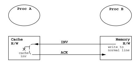
Figure 4: Normal invalidation is performed by hardware. Node *A* has cached a read copy of a memory line from Node *B*. When a write occurs, The hardware at Node *B* invalidates the read copy using messages generated and interpreted by hardware.
