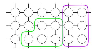
Figure 2: Two process groups scheduled together on separate nodes of the same multiprocessor.
