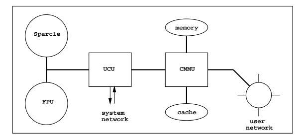
Figure 10: FUGU node architecture.
