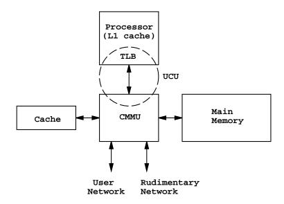
Figure 1: A FUGU node. The Communications and Memory Management Unit (CMMU) resides on the processor's external cache bus. The Translation Lookaside Buffer (TLB) is integrated with the processor. The User Communication Unit (UCU) refers to the set of hardware features that provide translation and protection for the hardware communication facilities.
