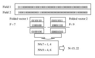
Figure 4. Multiple folding: Locating matching positions
