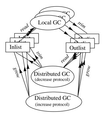
Figure 2-8: The roles of local and distributed GC in reference tracking
