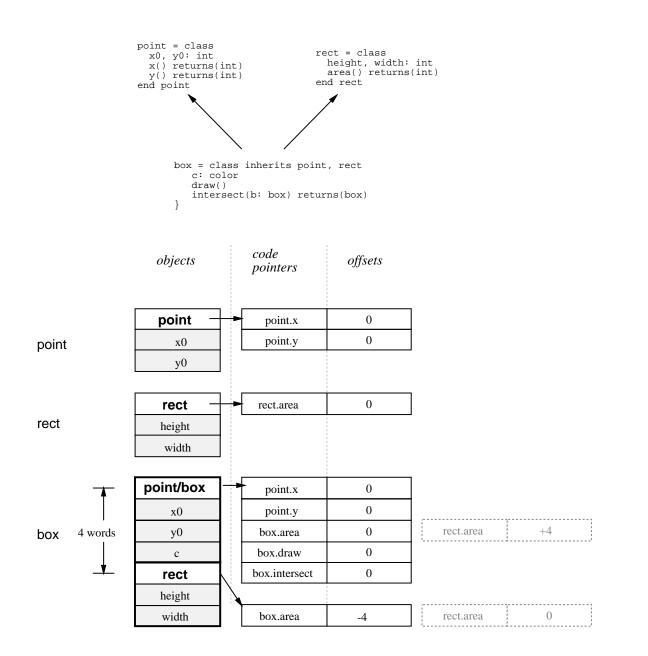
Figure 2-6: Pointer offsets in dispatch tables
