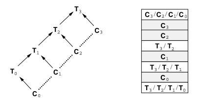
Figure 2-8: A class ladder and corresponding C++ object layout
