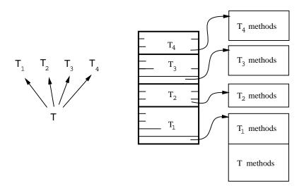
Figure 2-14: Recursively constructing type headers
