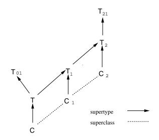
Figure 2-10: Supertypes and superclasses of a class
