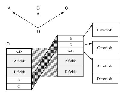
Figure 2-9: A C++ object with empty non-primary superclasses
