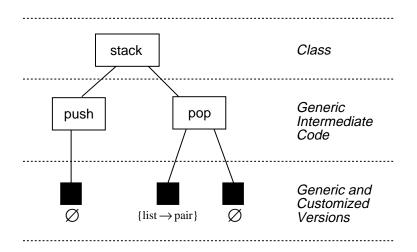
Figure 3-1: The information attached to methods
