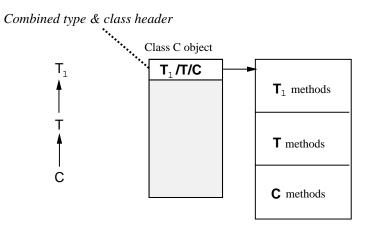
Figure 2-15: Result of merging type and class headers
