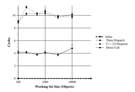
Figure 2-19: Call mechanism overhead on the MIPS R3000
