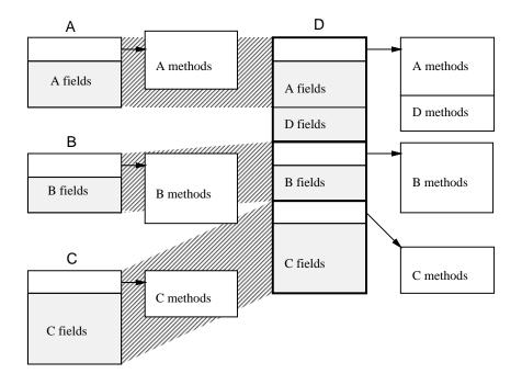
Figure 2-5: Multiple Inheritance with Embedded Objects
