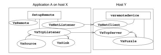
Figure 4.12: Remote Filter and Connections Setup
