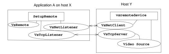
Figure 4.10: Remote Source and Connections Setup
