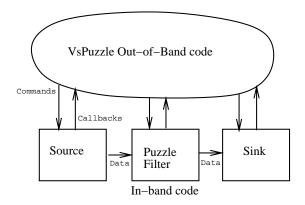
Figure 2.4: In-Band/Out-of-Band Partitioning in VsPuzzle
