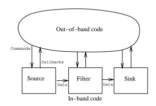
Figure 1.2: The structure of a simple VuSystem application
