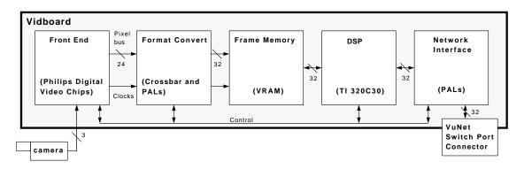
Figure 6: Block diagram of the Vidboard
