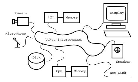
Figure 1: A Desk Area Network where devices are taken out of the workstation and attached directly to the network. The workstations coordinate the flow of data from various devices on the network to other devices.
