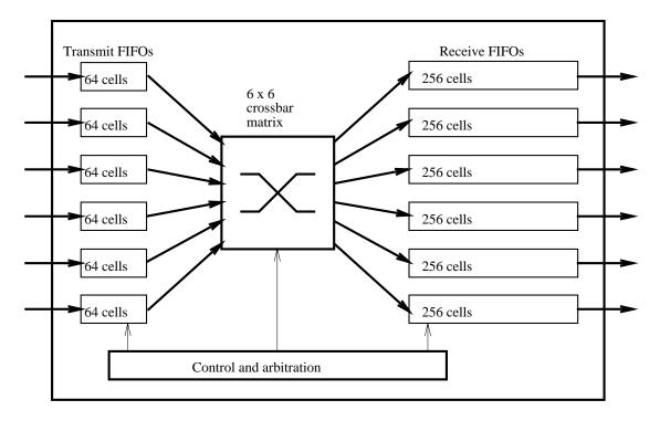
Figure 2: The six port VuNet switch.
