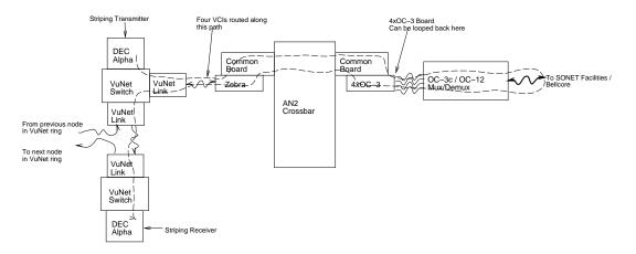
Figure 8: Environment developed for striping experiments.
