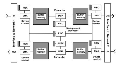
Figure 1: Block Diagram of High-Performance Flow Forwarder
