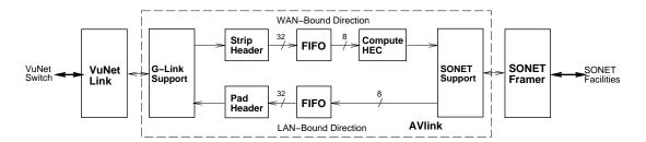
Figure 7: Block diagram of the AVlink
