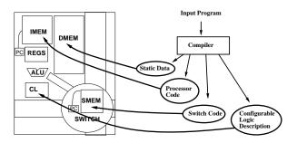
Figure 9: Compiler interaction with the architecture
