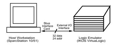
Figure 13: RawLogic: Prototype Reconfigurable Computing System
