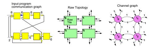
Figure 10: Input program communication graph, the Raw microprocessor topology, and the Raw communication channel graph showing the initial values of the available channel capacities.
