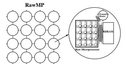
Figure 2: Raw multiprocessor comprising multiple Raw  $\mu$ Ps.
