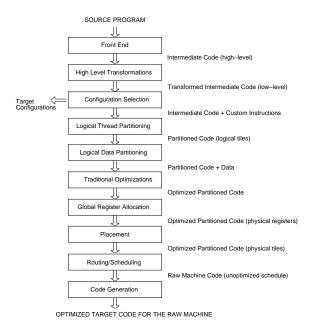
Figure 8: Compilation phases in Raw compiler
