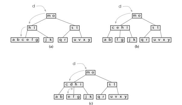
Figure 5. Single Insertion into a B-tree with s = 2
