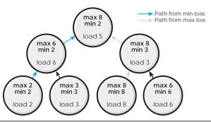
**Figure 8. Computing the Maximum and Minimum Loads**
