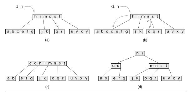
Figure 6. Bulk Insertion into a B-tree with s = 2
