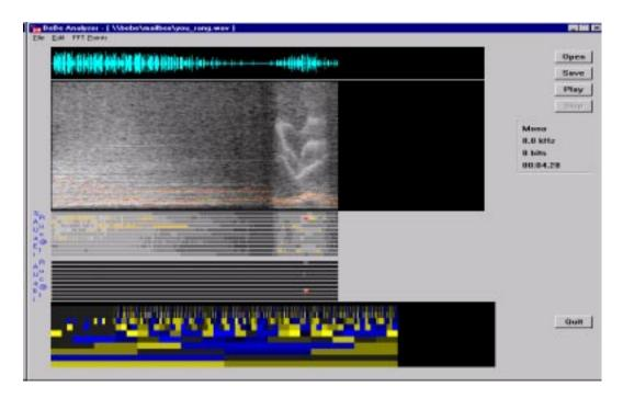
**Diagram 2.** A presentation of BeBe<sub>0</sub> at work. There are five display areas, from top to bottom: the waveform, the FFT spectrogram, the results from the detection algorithms, other information from the detection algorithms, and a wavelet transform.
