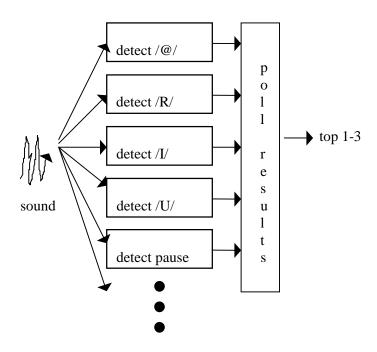
**Diagram 1**. Block diagram of BeBe System. The detection algorithms report the likelihood that the sound samples contain the designated phoneme. Examples of the sounds are: /@/ as in bat, /R/ as in stir, /I/ as in fit, and /U/ as in should.
