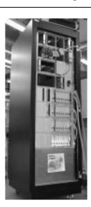
Figure 6-1: 16-node machine and 128-node chassis populated with a 32-node machine.
