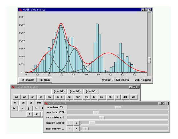
Figure 5-3: An interactive one-dimensional Gaussian mixture training tool.
