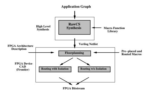
Figure 2-7: Frontier System Flow
