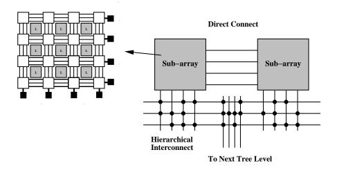
Figure 7-4: Partitioned Island-style Device
