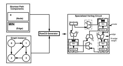
Figure 2-8: RawCS Flowchart for Shortest Path
