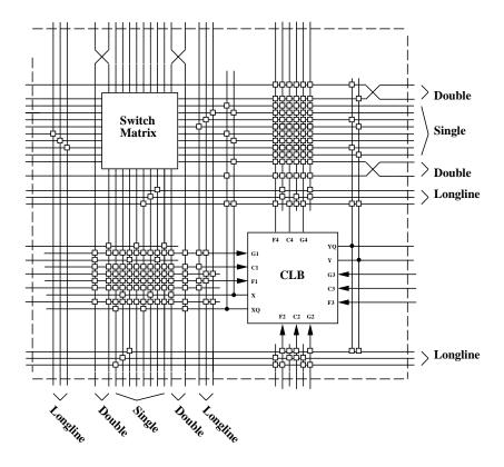
Figure 2-2: Xilinx XC4000 Routing Cell
