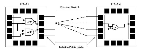
Figure 6-1: Isolation of Routing Resources
