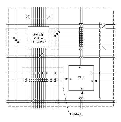
Figure 2-4: Thesis Routing Cell
