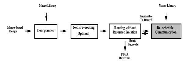
Figure 7-1: Design Flow with Communication Re-scheduling
