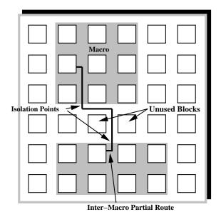
Figure 6-3: Planar Isolation Design Style
