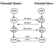
Figure 4. State transitions during the Page process.
