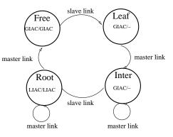
Figure 5. Node state transitions during topology construction. IACs used to transmit and listen during the Inquiry process are separated by /.
