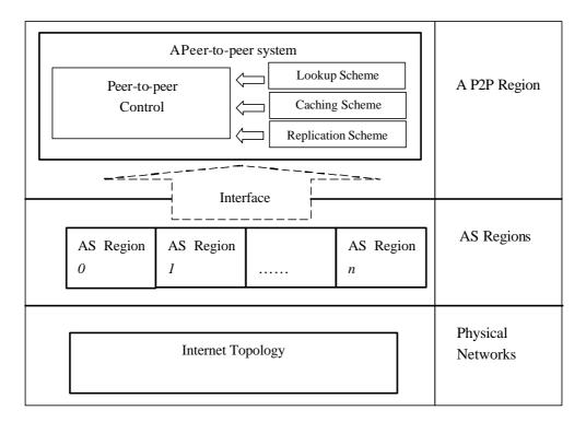
Figure 5.1: System Architecture
