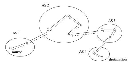
Figure 4.8: The caching algorithm
