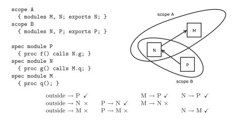
Fig. 13. Example of permissible inter-scope method calls
