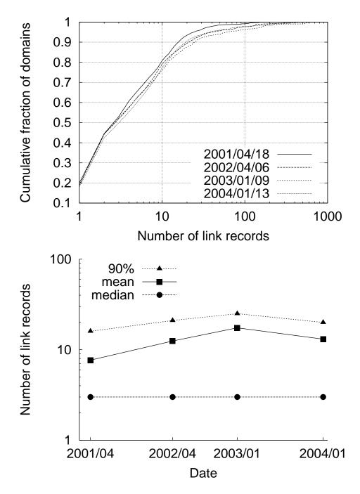
Figure 7-5: The number of link records in an edge domain's main topology database as a cumulative distribution, and the mean, median, and the 90th percentile.
