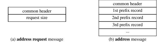
Figure 4-11: Contents of an **address request** message and an **address** message.
