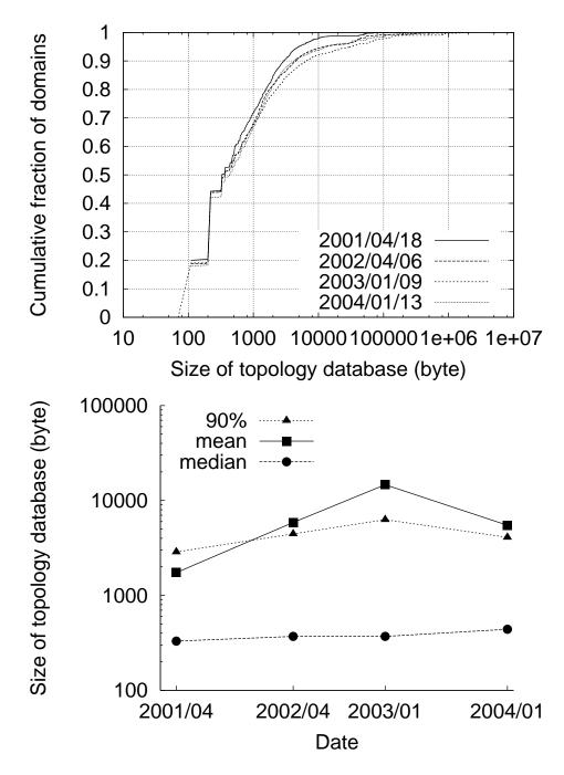
Figure 7-6: The size (in byte) of an edge domain's main topology database as a cumulative distribution, and the mean, median, and the 90th percentile.
