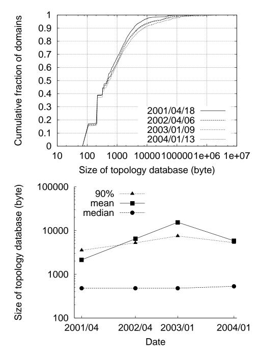
Figure 7-4: The size (in byte) of a domain's main topology database as a cumulative distribution, and the mean, median, and the 90th percentile.
