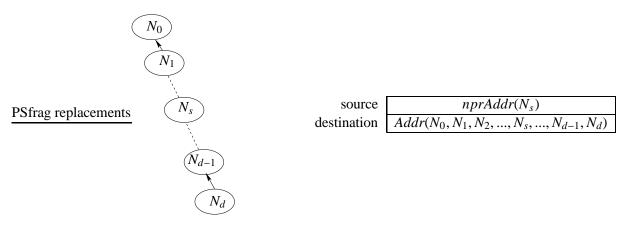
Figure 5-17: This figure shows a downhill route segment and its representation.
