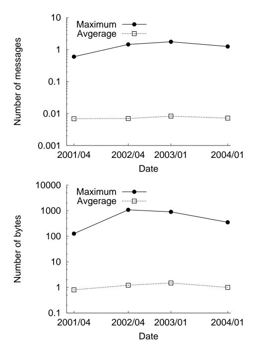
Figure 7-9: The average and maximum number of messages and bytes sent per failure per link.
