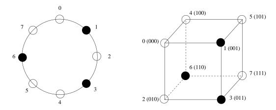
Figure 2-6: An example of the ring geometry and the hypercube geometry for an identifier space of size 8. A circle represents the position of an identifier in a geometry, and a filled circle represents an identifier taken by a node.
