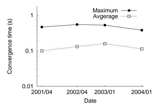
Figure 7-10: The average and maximum time elapsed between the time a failure is detected and the time the last topology message triggered by the failure is received.
