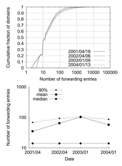
Figure 7-7: The number of forwarding entries in a TIPP router's three logical forwarding tables as a cumulative distribution, and the mean, median, and the 90th percentile.
