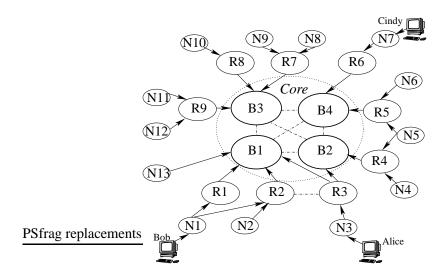
Figure 3-1: A simplified view of the Internet domain-level topology. A domain is represented by an ellipse. An arrowed line between two domains represents a provider-customer connection, with the arrow ending at the provider. A dashed line represents a peering connection.
