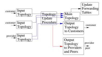
Figure 4-15: When a router receives a **topology** message from a neighbor, it first updates the input topology database for the neighbor. If the input topology database is connected to the output topology database of a neighbor class, the router will invoke the topology update procedure and send changes to the corresponding neighbors. The router may also update its forwarding tables.
