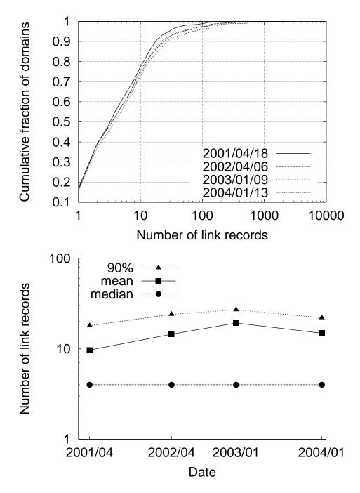
Figure 7-3: The number of link records in a domain's main topology database as a cumulative distribution, and the mean, median, and the 90th percentile.
