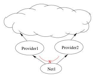
Figure 2-7: Packets are generally forbidden to traverse the path Provider1  $\rightarrow$  Net1  $\rightarrow$  Provider2. An arrowed line in the figure represents a customer-provider connection, with the arrow ending at the provider.
