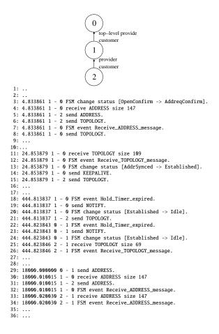
Figure 4-17: Each line shows a TIPP event happened at a simulated time point. The notation i - j means node *i*'s connection to a neighbor *j*.
