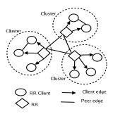
Figure 1. iBGP using route reflection
