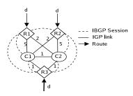
Figure 3. An iBGP configuration using route reflectors that has low fault tolerance
