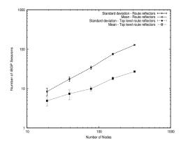
**Figure 9.** Number of route reflectors vs n - AS1239
