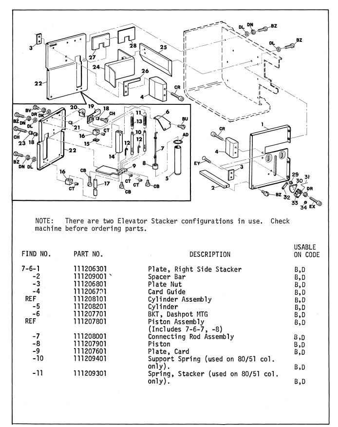
FIGURE 7-6 ELEVATOR STACKER ASSEMBLY
