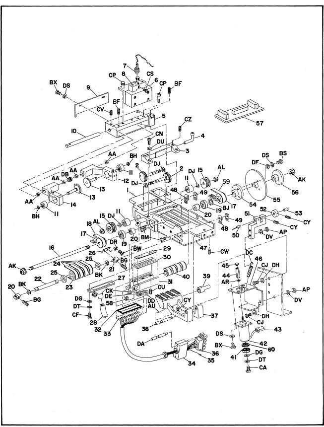
FIGURE 7-2 EXPLODED VIEW PICKER, PICKER SOLENOID AND READER ASSEMBLY
