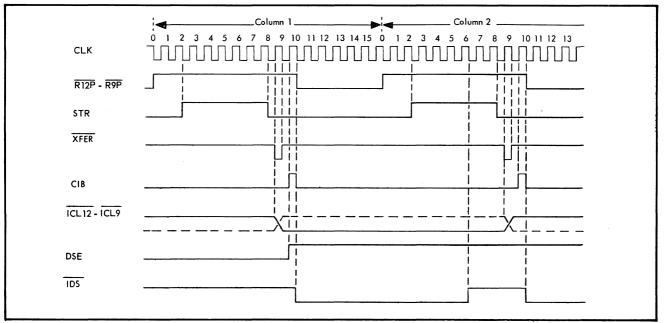
FIGURE 4-2 READ TIMING DIAGRAM
