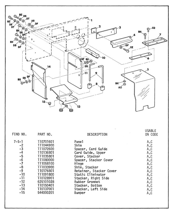
FIGURE 7-5 GRAVITY STACKER
