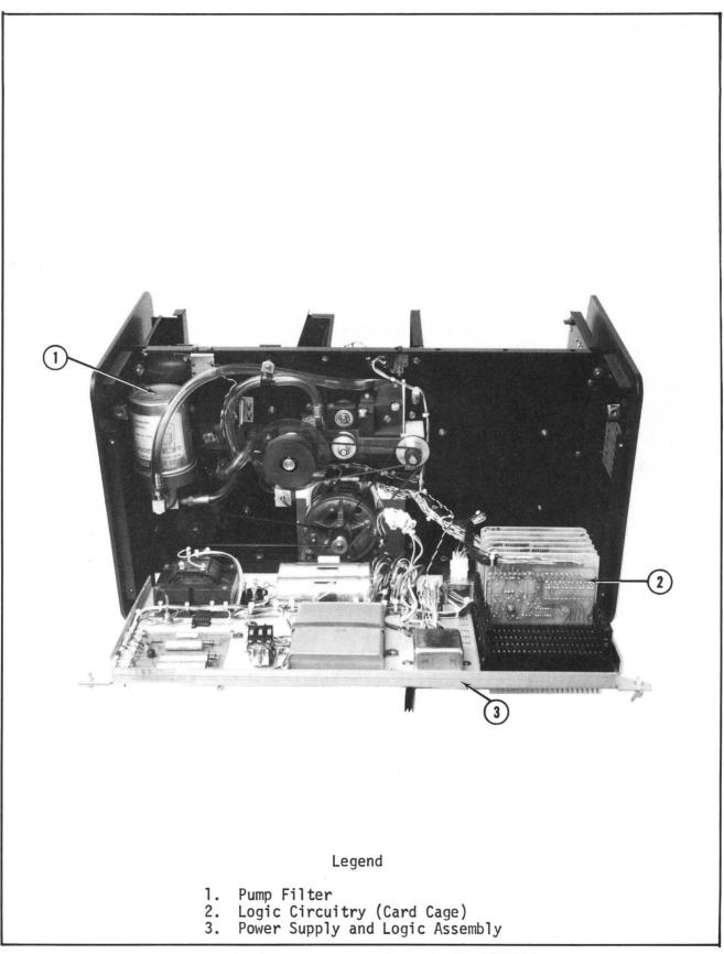
FIGURE 5-3 HINGED CHASSIS OPEN, 6002/6002A
