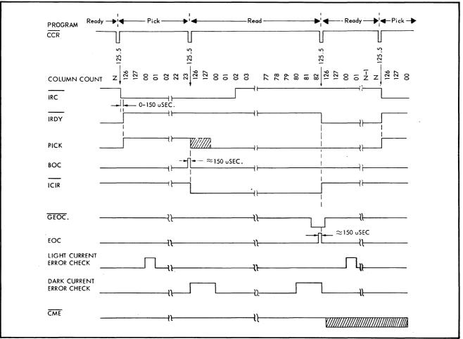
FIGURE 4-1 FEED TIMING DIAGRAM
