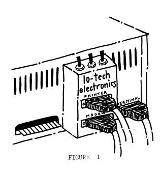
of the pins is mirror-imaged between the two connector types so that when they are plugged together everything hooks up properly. Your pin requirements may differ; you may have to switch lines 2 and 3 for output to the modem (see Appendix D of your MD manual) or you may not need all nine lines.
