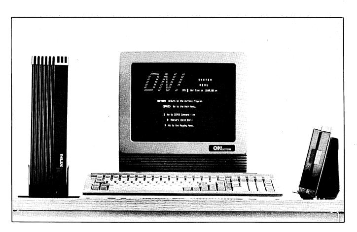
its built-in power protection, which has two stages. First, the ON! has all the protection from spikes, dips, and electrical noise you could want built in--well beyond that supplied by most surge suppressors and other add-on devices. The ON! also has filtered power outlets on its back panel so that you can plug in the terminal and other electrical equipment to take advantage of the ON!'s protection.
