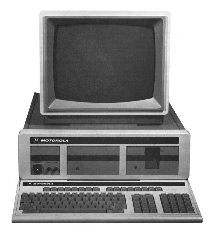
FIGURE 1-1. VME/10 Microcomputer System
