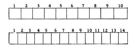
b. The **Input** Register is initially filled by the READ CARD command with a group of digits which are inserted into the corresponding digit positions of the proper words in the Buffer Register when signals are received at the inlet hubs. The  $\frac{1}{1000}$  register is indexed by the <del>sidend</del> register as each row of the card passes under the reading brushes so that holes in each succeeding row insert the next value into the Buffer Register.
