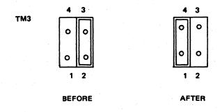
Figure 7 TM3 Jumper Position
