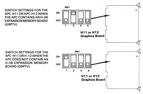
Figure 9 Switch Positions for the APC-H11/H12
