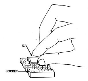
Figure 5 Inserting the IC into the Socket
