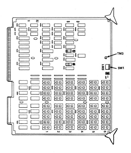
Figure 6 TM3 Jumper Location on the APC-H31 PCB Revision 1
