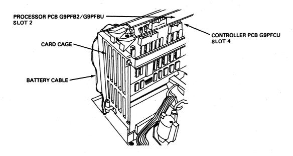
Figure 11 Card Cage (Front View)
