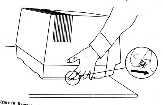
Figure 10 Removing the APC Top Cover
