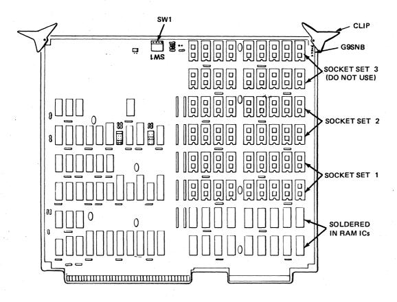
Figure 1. The APC-H31 Memory Expansion Unit PCB (G9SNB)
