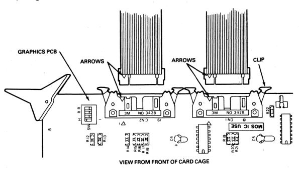
Figure 12 Disconnected Cables
