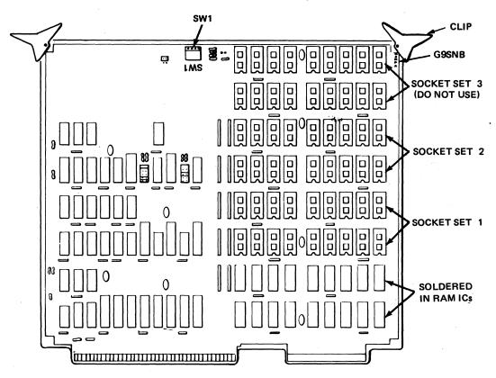
Figure 4 The APC-H31 Memory Expansion Unit PCB (G9SNB)
