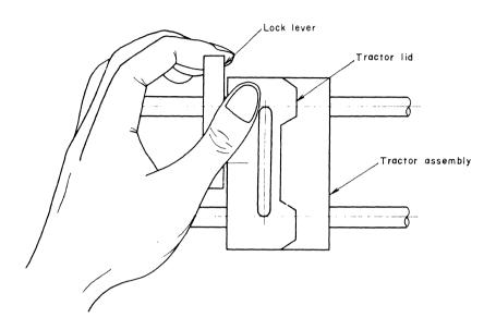
(2) Push the lock lever with your thumb to lock the tractor, while supporting the shaft with your other fingers.
