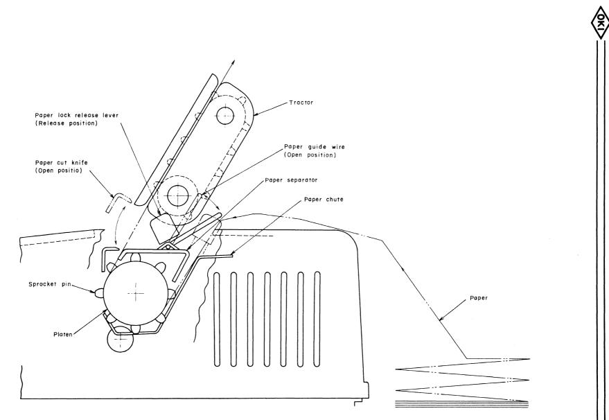
Fig. 3-7 Fixed Sprocket Paper Loading Method
