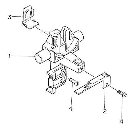
Fig. 7-7 Carriage Assembly (5LR-129865)
