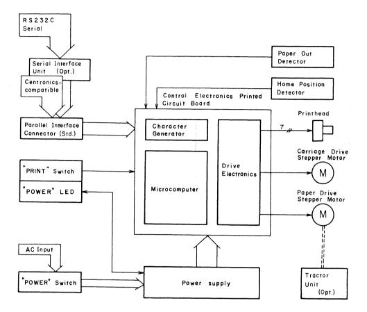
Fig. 1-1 Block Diagram
