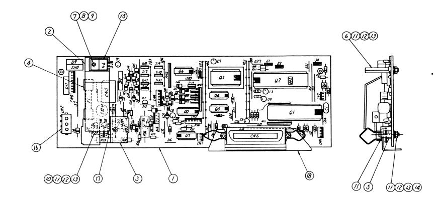
Fig. 7-11 LEPU Circuit Board (2LX-86695)
