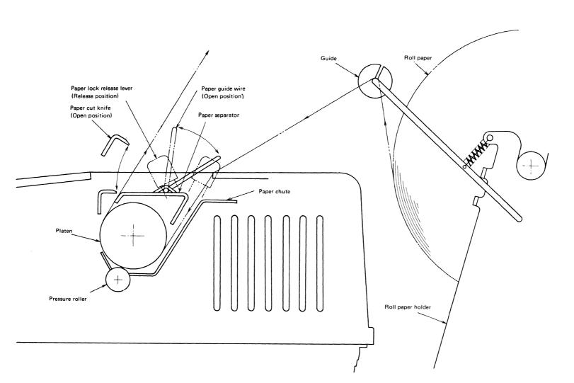
Fig. 3-5 Roll Paper Loading Method
