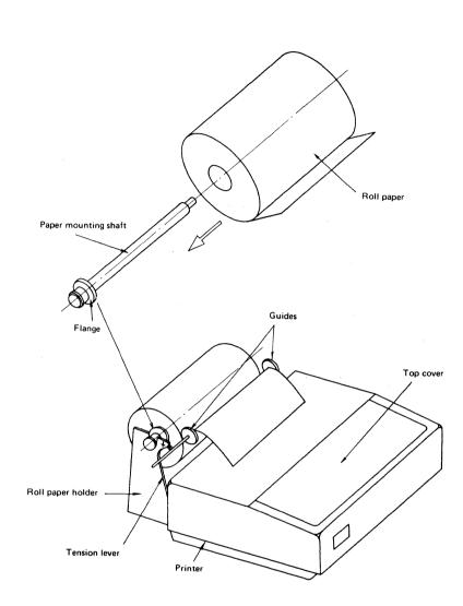
Fig. 3-4 Roll Paper Loading Method
