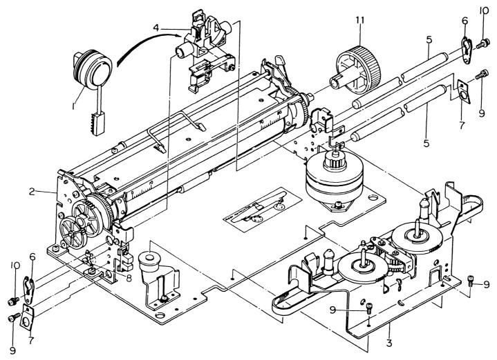
Fig. 7-2 Printer Unit (2LR-1322-2)
