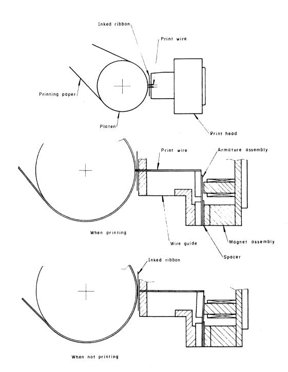
Fig. 4-1 Printing Mechanism
