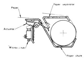
Fig. 4-6 Paper End Detecting Mechanism
