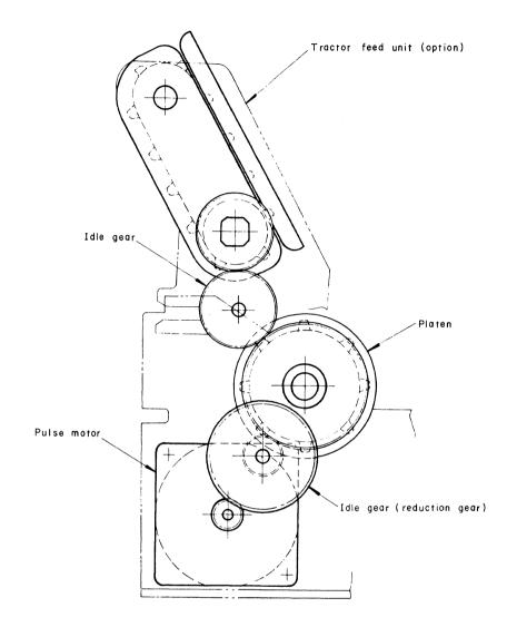
Fig. 4-4 Paper Feed Mechanism
