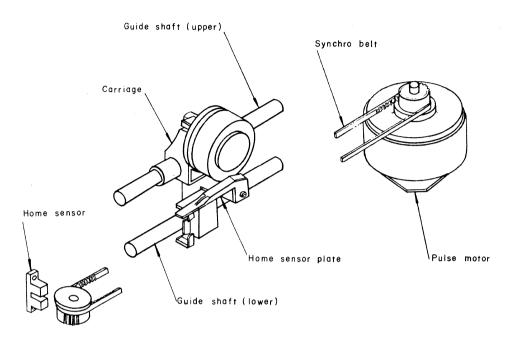
Fig. 4-2 Spacing Mechanism
