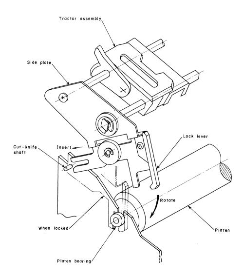
Fig. 3-2 Tractor Unit Installation
