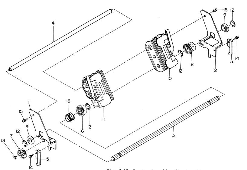
Fig. 7-12 Tractor Assembly (2LR-129880)
