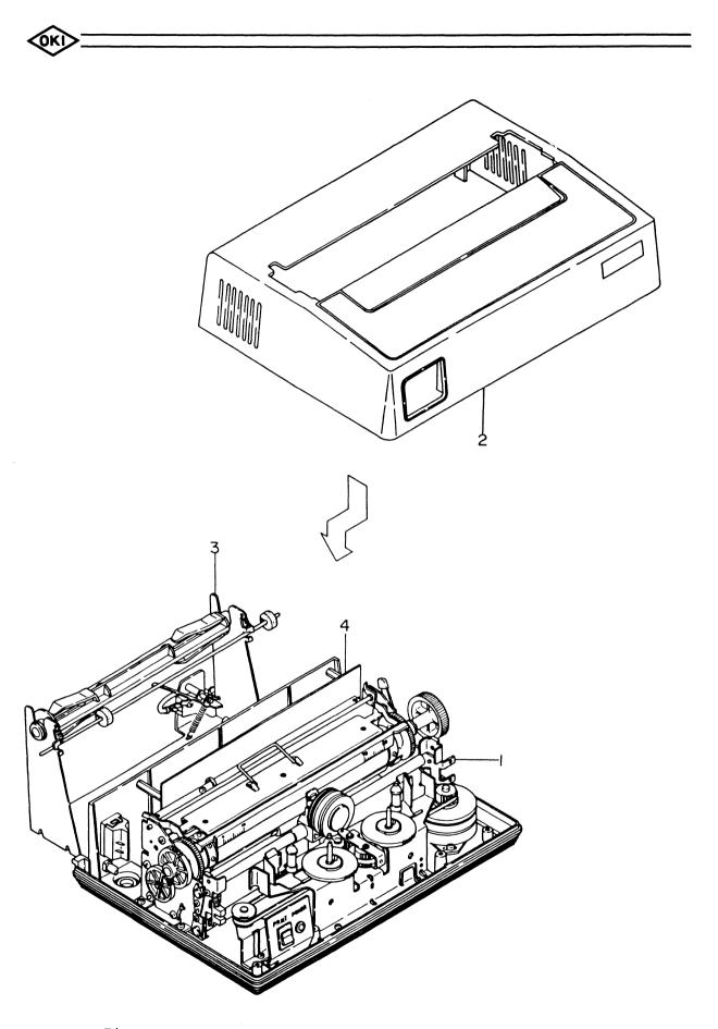
Fig. 7-1 General Assembly Diagram (LY-43204-3, 4) (1/2)
