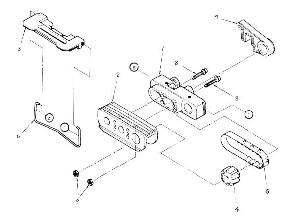
Fig. 7-13 Sheet Feeder Assembly (R) (FMX-35100-2)
