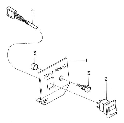
Fig. 7-9 Switch Assembly (5LM-58646)
