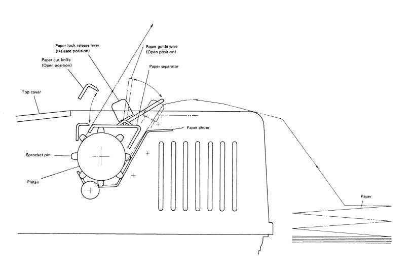
Fig. 3-6 Fixed Sprocket Paper Loading Method
