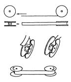
(4) Mount one ribbon spool on the spool shaft. Make sure that the winding direction is as shown in Fig. 3-6, and that the ribbon drive pin is in the spool hole.
