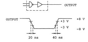
The above values apply for a drive source voltage of  $\pm 12$  V, and a 7  $k\Omega$  , 15 pF load.
