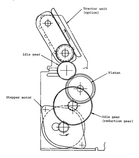
Fig. 5-4 Paper Feed Mechanism
