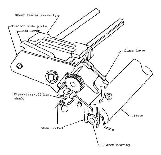
Fig. 3-4 Tractor Unit Mounting Method
