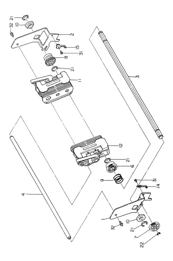
Fig. 8-14 Tractor Unit (LY-37539)
