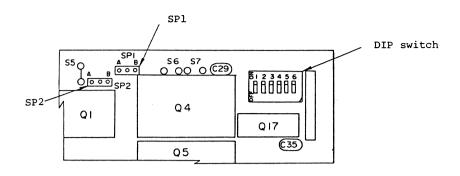
Fig. 4-3 DIP Switches and Jumper Plugs on Control Circuit Board
