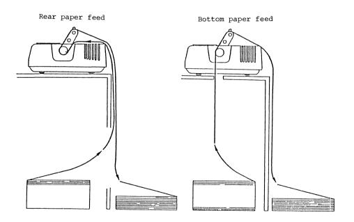
Fig. 3-8 Sprocket Paper Positioning
