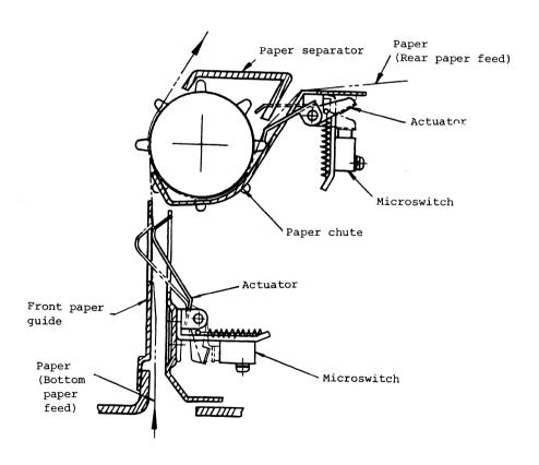
Fig. 5-6 Paper Out Detecting Mechanism
