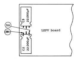
The circuit is so designed that the rated currents may flow through the motors and magnet even if the 35 V fluctuates due to input voltage fluctuation and load fluctuation.
