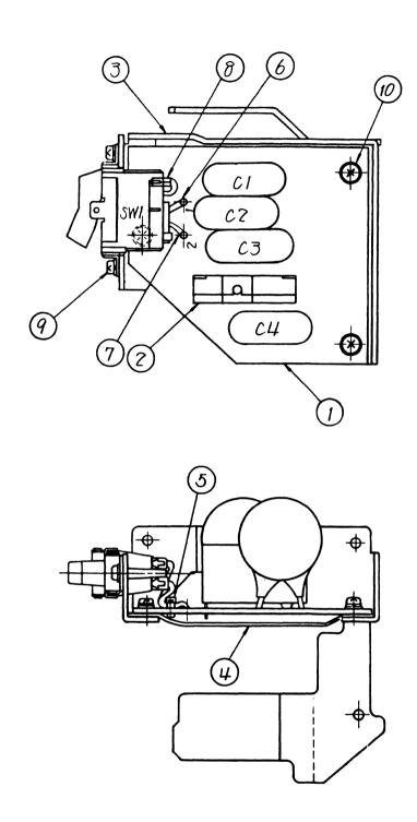
Fig. 8-12 LEPW-1 Circuit Board Assembly (3LX-86727-1) (for 115 V)
