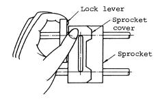
When locking the sprocket lock lever, push the lock lever with your thumb while holding the shaft with the other fingers.
