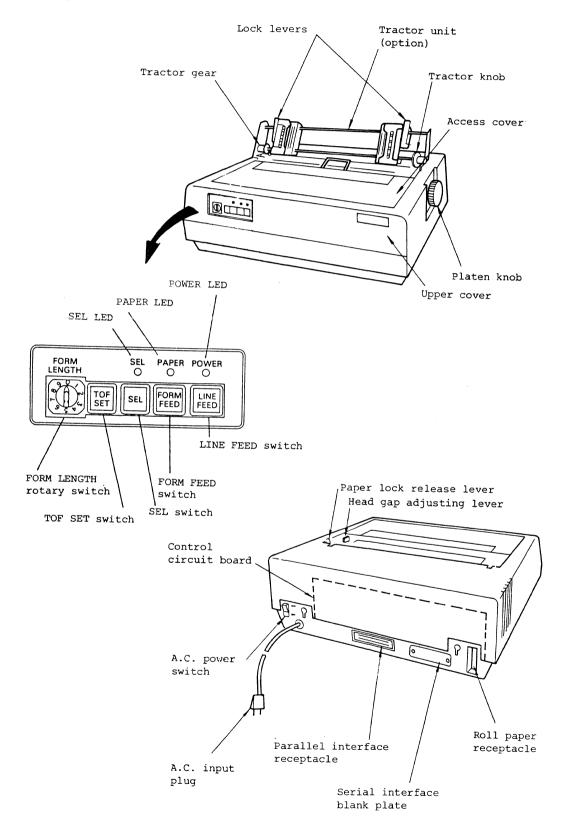
Fig. 3-3 Operating Controls, LEDs and Others
