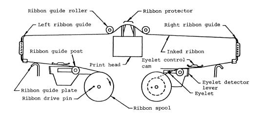
Fig. 3-6 Ribbon Loading Method
