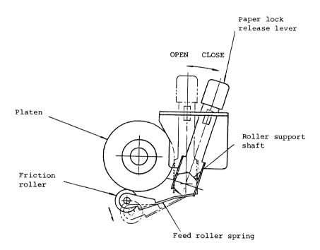
Fig. 5-5 Paper Lock Release Mechanism
