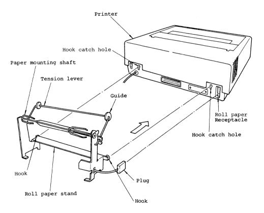
Fig. 3-5 Roll Paper Stand Mounting Method
