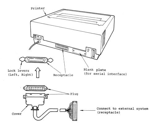
Fig. 3-1 Parallel Interface Connection Diagram
