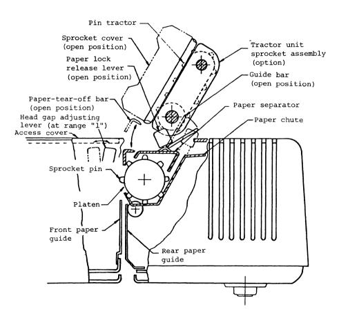
Fig. 3-7 Sprocket Paper Loading Method
