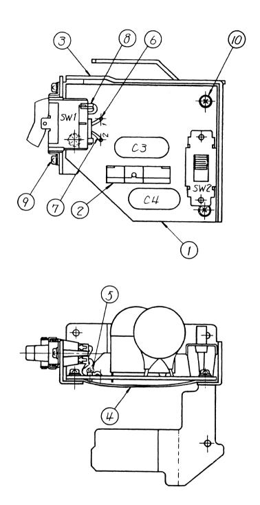
Fig. 8-12 LEPW-2 Circuit Board Assembly (3LX-86727-2) (for 220/240 V)
