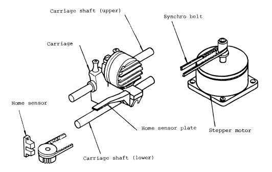
Fig. 5-2 Spacing Mechanism
