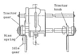
(5) For bottom paper feed, slide the paper up from the bottom frame hole, between the front paper guide and the rear paper guide and fit the paper sprocket holes over the sprocket pins of the platen and of the sprocket on the tractor.
