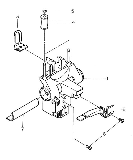
Fig. 8-7 Carriage Assembly (4LR-191870)
