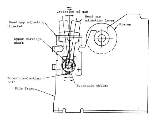
Fig. 5-7 Head Gap Adjusting Mechanism
