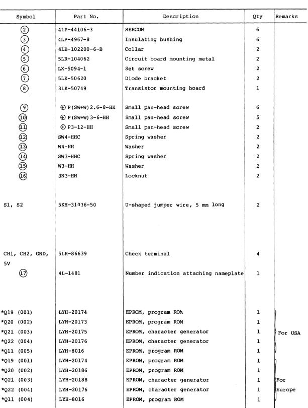
Figure 9-14 HLPA Circuit Board Assembly (LY-43360) 4/4 (2nd edition)
