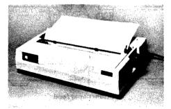
The cut-sheet paper loading procedure is now complete. Note: Cut-sheet paper cannot be used if the tractor unit is installed.
