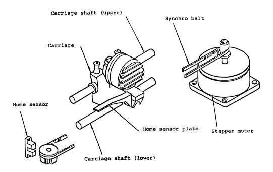
Figure 6-2 Spacing Mechanism
