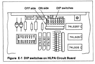
Functions in the tables below can be selected by setting and combinations of DIP switches on PC board. The DIP switch names and numbers are indicated on PC board by silk-screen print.
