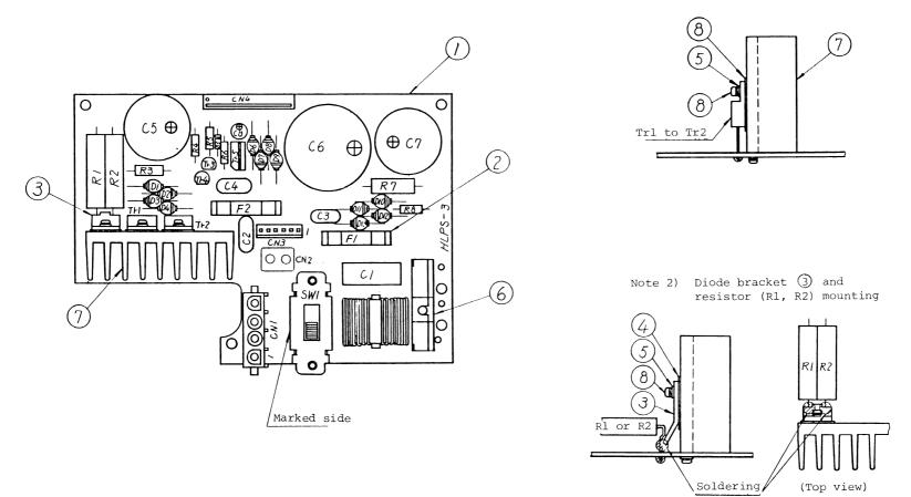
Figure 9-12 HLPS-3 Cirbuit Board Assembly (LY-43361-3) (for Europe) (2nd edition)
