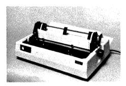
(5) For bottom paper feed, slide the paper up from the lower cover hole, between the front paper guide and the rear paper guide and fit the paper sprocket holes over the sprocket pins of the platen and of the sprocket on the tractor.
