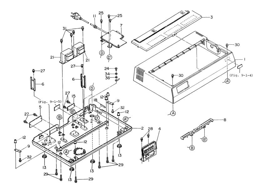
Figure 9-8 Cover Unit (1LM-61285-3) (for Europe)(for 220/240 V)
