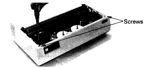
(6) Lift the front upper cover, tilt backward, and lift from the lower cover.
