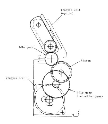
Figure 6-4 Paper Feed Mechanism
