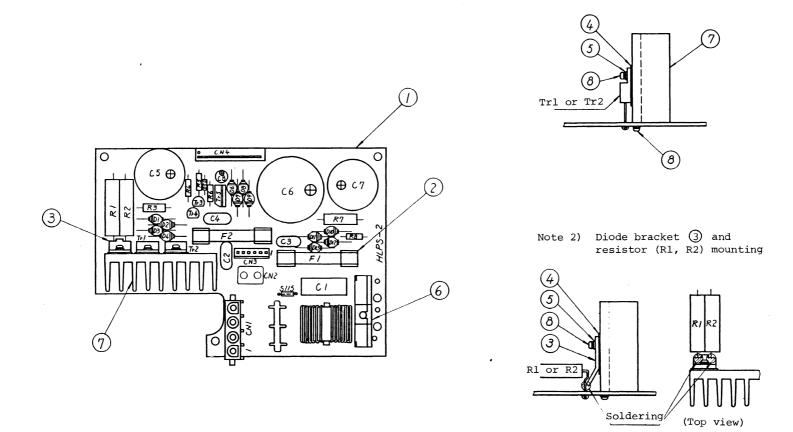
Figure 9-12 HLPS-2 Cirbuit Board Assembly (LY-43361-2) (for USA) (2nd edition)
