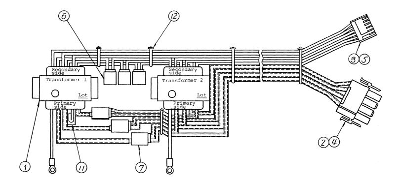
Figure 9-13 Transformer Assembly (2LR-192189-3) (for Europe) (2nd edition)
