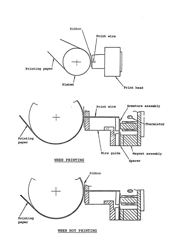
Figure 6-1 Printing Mechanism
