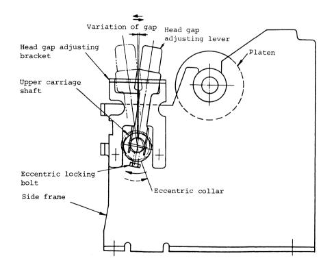
Figure 6-7 Head Gap Adjusting Mechanism
