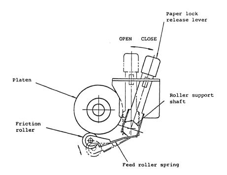
Figure 6-5 Paper Lock Release Mechanism
