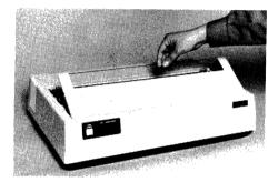
(5) Remove the screws on each side of the upper cover.
