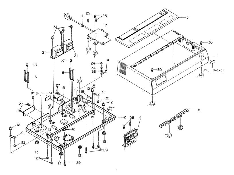
Figure 9-8 Cover Unit (1LM-61285-2) (for USA) (for 115 V)
