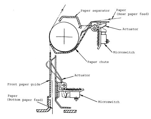
Figure 6-6 Paper Out Detecting Mechanism
