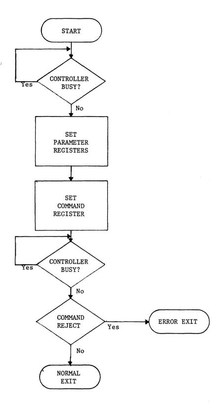
Figure 1. Basic Command Flow
