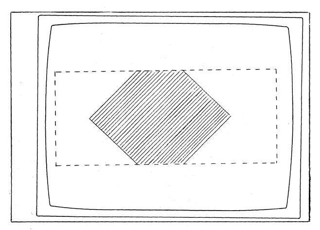
Figure 3.2c Polygon in Smaller Clipping Window
