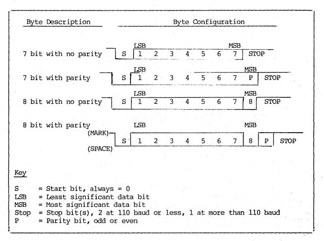
Figure 13.3 Model One/10 Byte Configurations
