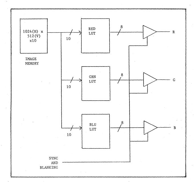
Figure 8.1 Image Memory Output Diagram
