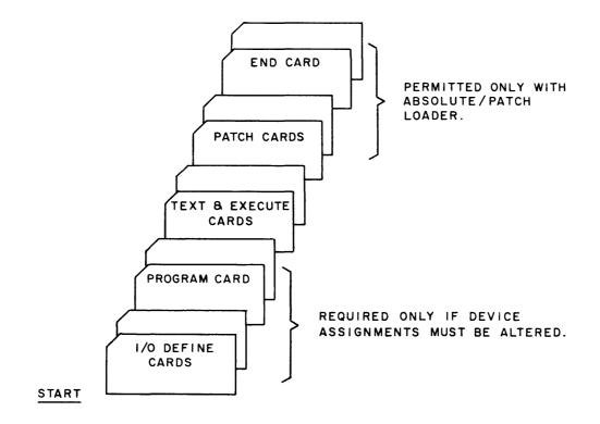
Figure 8. Absolute Card-Deck Load
