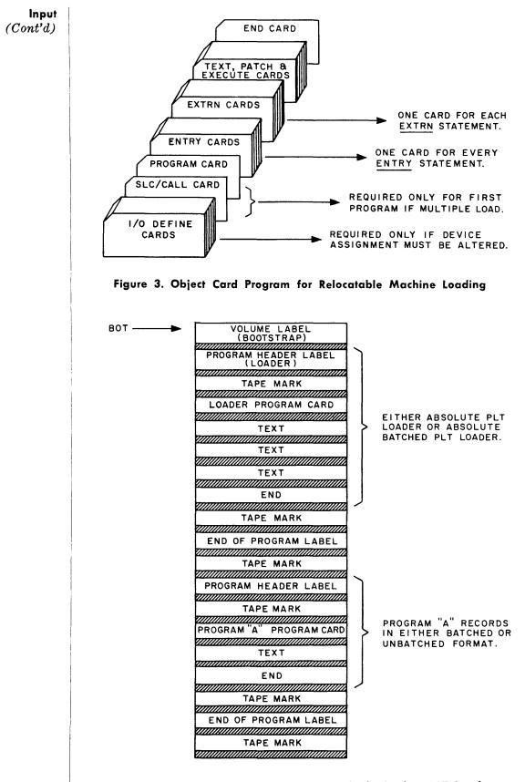
Figure 4. PLT Used by Absolute and Batched Absolute PLT Loaders
