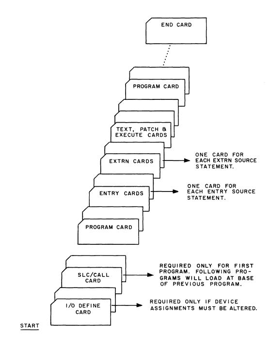
Figure 9. Relocatable Card-Deck Load
