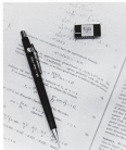
Microsil depicts 8087 made by National Semiconductor, the specialized type of processor, called a floating-point processor, or co-processor, made to do all math calculations.
