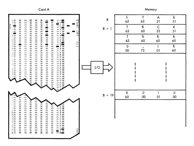
Figure 4-4. Card Read Into Memory in Hollerith
