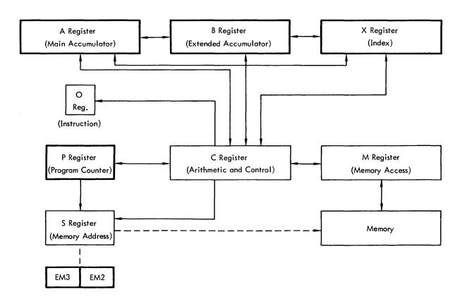
Figure 1-2. Basic Register Flow Diagram
