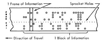
The organization of information on the tape is in blocks. A block is a group of frames set off by a gap of at least one blank frame (in which only the sprocket hole is punched) at either end. Blocks may be of variable lengths.
