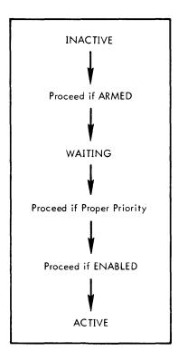
Figure 3-1. Interrupt Arm-Enable Response
