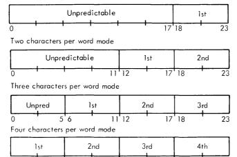
The unfilled character positions contain unpredictable data. When assembled during a single-word operation, a WIM instruction places the word into memory. Under interlace control,
