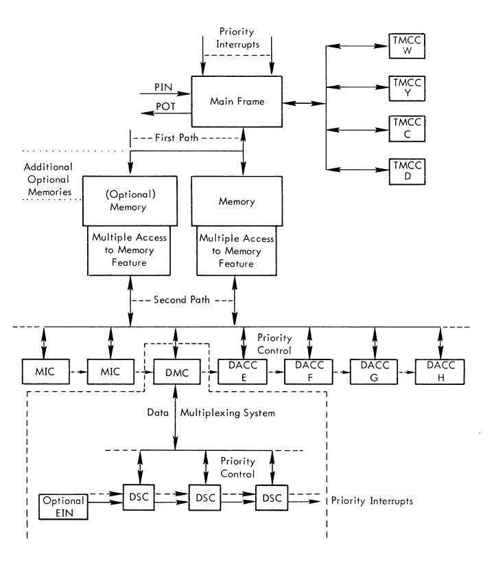
Figure A-1. XDS 930 Overall Computer Configuration
