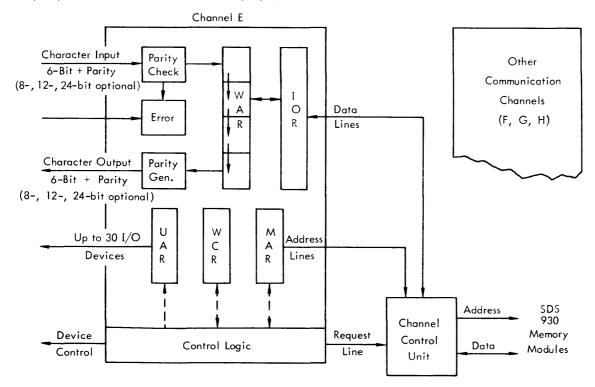
Figure 4-2. XDS 930 Direct Access Communication Channel, Block Diagram
