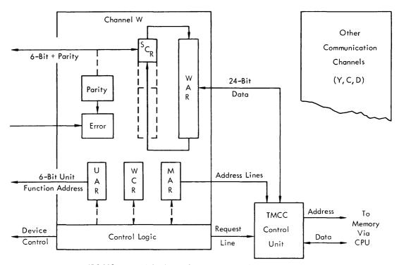
Figure 4-1. XDS 930 Time-Multiplexed Communication Channel, Block Diagram
