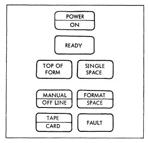
Figure 4-5. Printer Control Indicator Lights and Switches
