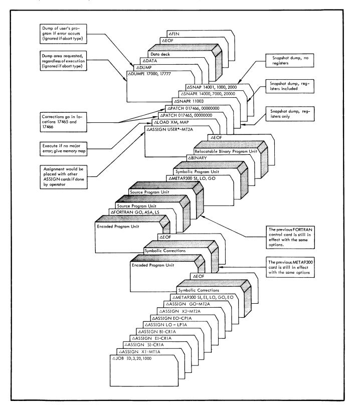
Note that when the Monitor encounters a FORTRAN or META-SYMBOL card, control is transferred to the appropriate processor immediately after the Monitor sets up the requested options. If any control card immediately followed the FORTRAN or META-SYMBOL card, or were within the source deck, it would cause an End-of-File exit from the processor-called I/O routine back to the Monitor; thus, the job would be aborted.
