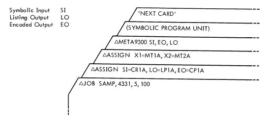
This setup has the name SAMP, account number 4331, time estimate 5 minutes, output estimate 100 pages, and assignment use of (from Monitor's standard assignments): Symbolic input from card reader 1 on channel A; listing output on line printer 1 on channel A; and encoded output on card punch 1 on channel A.
