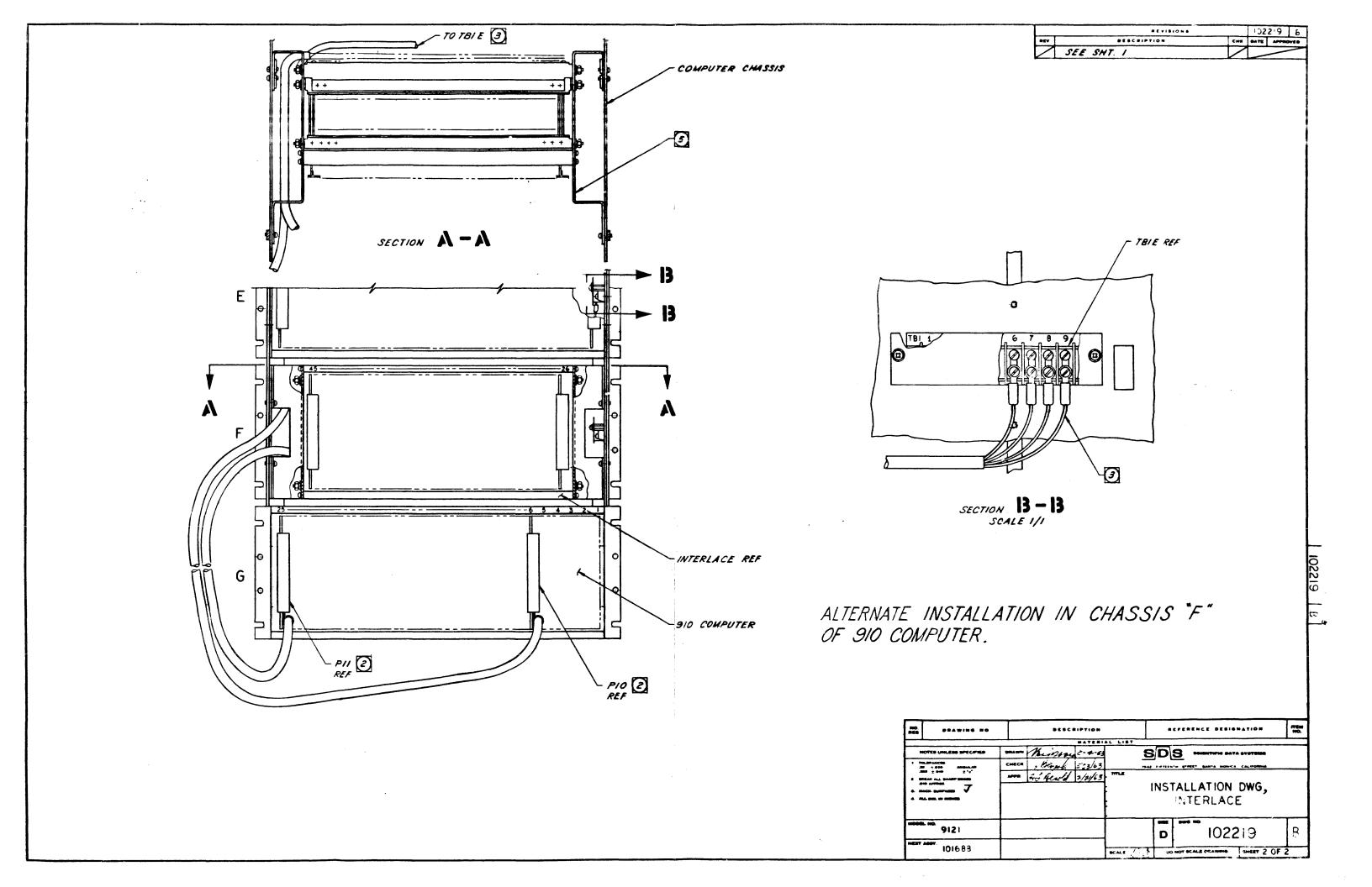
1. If unit is to be a "W" Interlace, remove the following wires:
