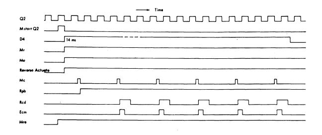
Figure 6. Magnetic Tape Erase, 41.7 Kc, Initial Start Reverse
