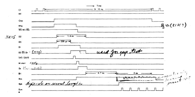
Figure 9. Magnetic Tape Write, 41.7 Kc, Forward Continue
