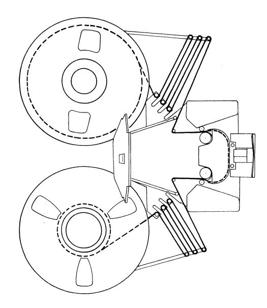
Figure 3. Magnetic Tape Threading Procedure, Potter MT-120
