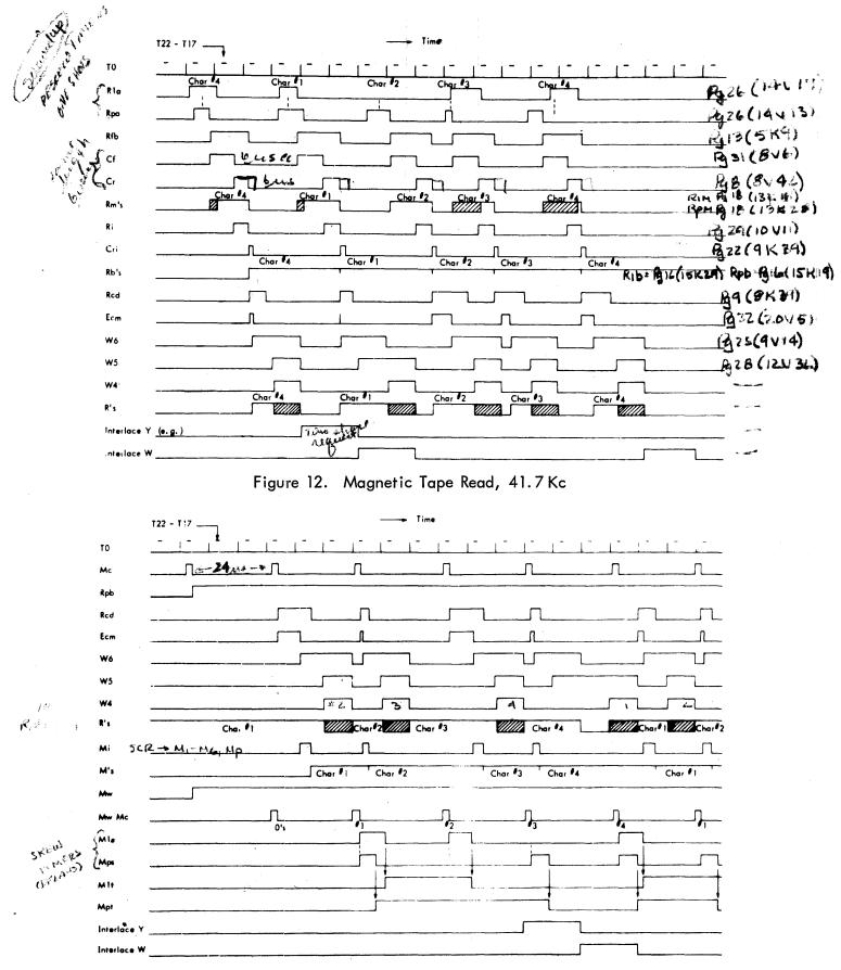
Figure 13. Magnetic Tape Write, 41.7 Kc
