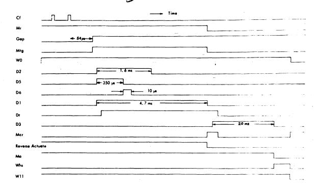
Figure 8. Magnetic Tape Read, 41.7 Kc, Reverse Operation Termination
