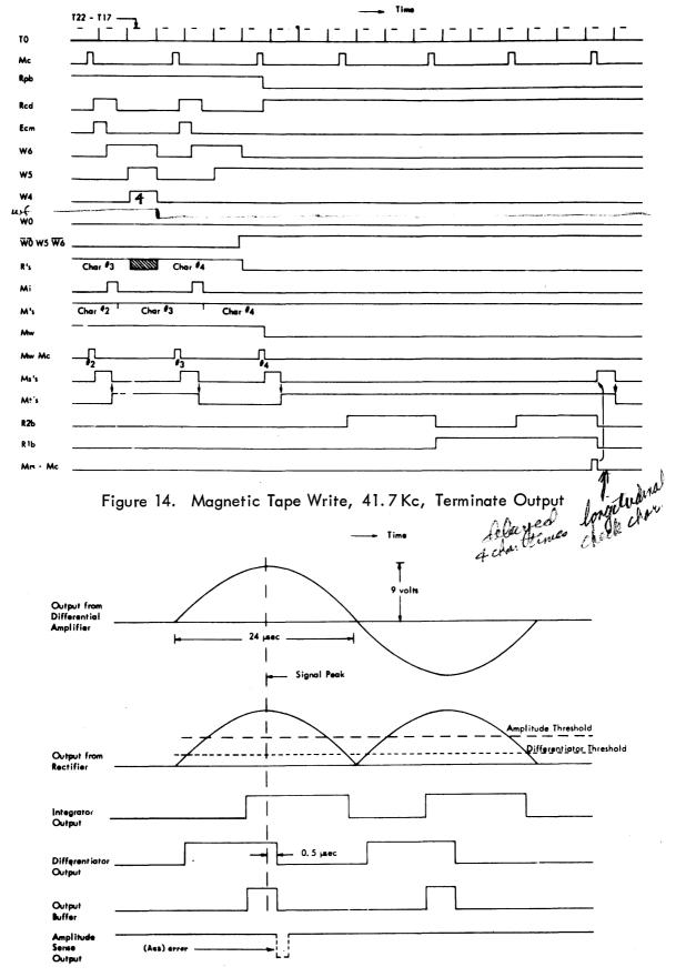
Figure 15. Magnetic Tape Read, 41.7 Kc, Read Amplifier Signals
