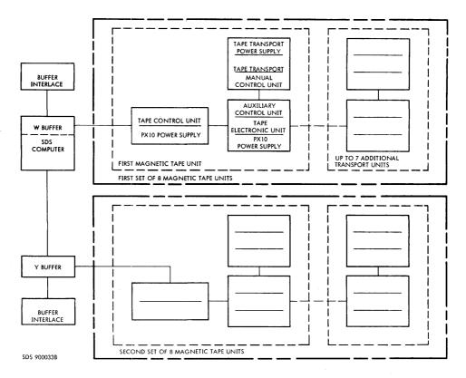
Figure 1. Magnetic Tape System Configurations
