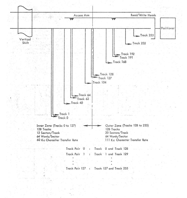
Figure 6. Organization of Model 9165 Inner/Outer Recording Zones and Track Pairs
