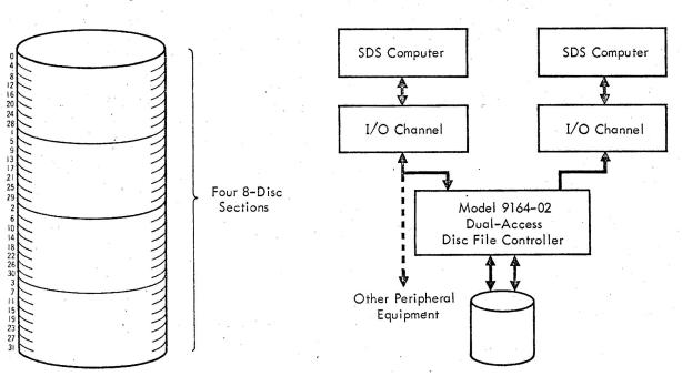
Figure 1. Disc Numbering — For programming purposes, the discs are numbered so that 0-3, 4-7, ..., 28-31 reside in four different sections of the file Figure 2. Two SDS Computers Sharing a Dual-Access Disc File System
