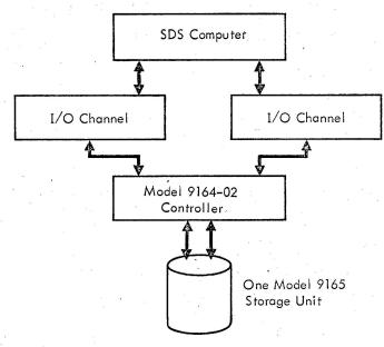
Figure 3. One SDS Computer with Dual Operation of File Storage Unit
