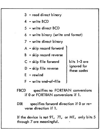
Figure 17. I/O Operation Codes for Device Handler (M:QUE) (cont.)
