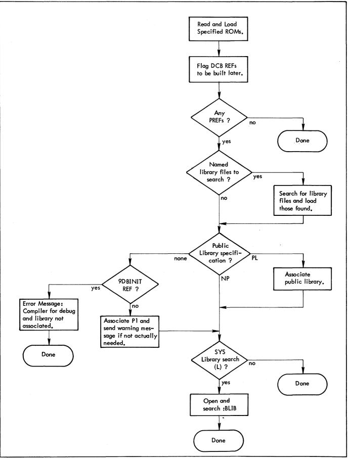
Figure 14. Generalized Library Load Process (Link)
