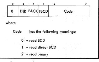
Figure 17. I/O Operation Codes for Device Handler (M:QUE)
