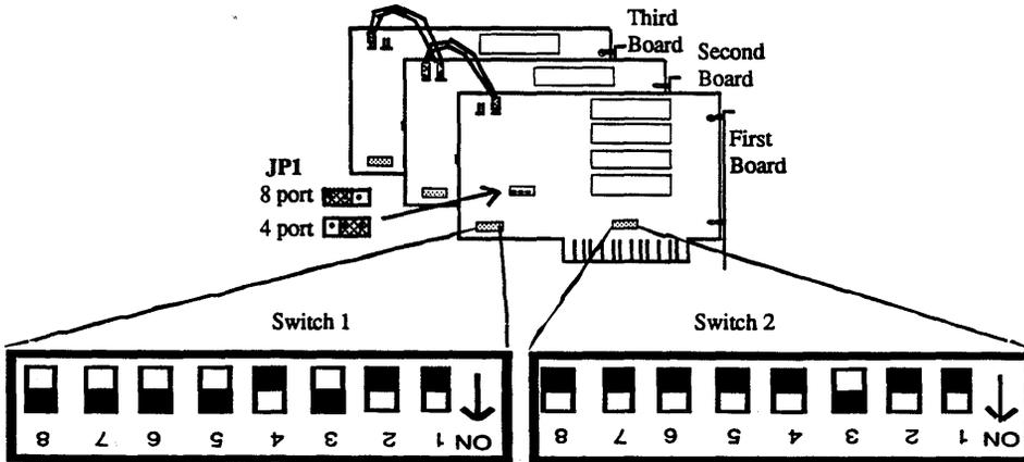
Switch 1 sets the I/O addresses for the card. The example above shows the setting for I/O address 140h. Each adapter in the system needs to have its own unique I/O address setting (see below).
