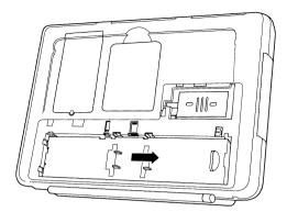
**6.** Replace the battery compartment cover. If the battery compartment cover is not replaced completely, the unit will not power on.
