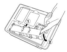
**3.** Install 6 AA-size alkaline batteries into the main battery case carefully, observing the correct polarity as shown below.
