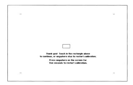
Touch in the rectangle to check if the calibration is successful. If you failed, the system asks you to repeat the process from the beginning.
