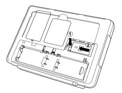
**5.** Remove the old lithium batteries and install two new lithium batteries (CR2032) of the same type. Place one into the left slot with the – side down and one into the right slot with + side down.
