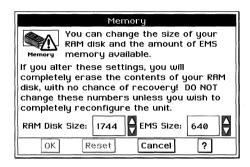
**3.** Set the RAM Disk Size value by tapping the up or down arrow button on the right of RAM Disk Size: box. The value increases or decreases by 16. The EMS size is increased or decreased automatically depending on the RAM Disk Size value.
