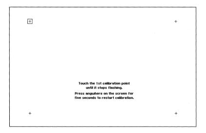
This procedure calibrates the unit to recognize the position on the screen which the pen touches. Tap the center of the flashing cross on the upper left of the screen gently. In the same way, tap the crosses on the upper right, lower left, and lower right of the screen. The following message appears:
