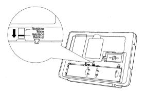
**4.** Hold down the latch which secures the backup battery cover (①), and slide the cover toward the latch (②), then remove it.
