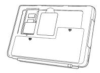
**4.** With the connector on the memory card facing down, push it firmly until the connectors on the memory card and in the compartment fully mate.
