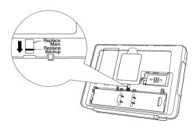
**2.** Hold down the latch which secures the backup battery cover (①), slide the cover toward the latch (②), then remove it.
