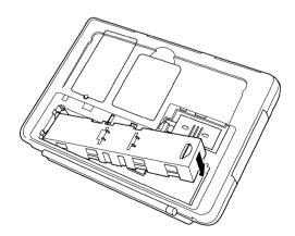
5. Slide the battery case in until the main battery lock clicks.
