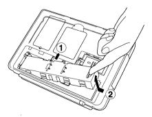
**5.** Place a lithium-ion battery in each side of the main battery slot. Make sure the arrow mark on the top of each battery points toward the outside.
