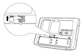
**4.** While sliding the main battery lock to "Release" (①), remove the main battery case by hooking a finger into the groove on the top of the battery case (②).
