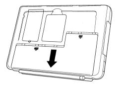
3. Slide the battery protect switch to "Replace Main".
