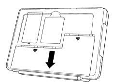
3. Slide the battery protect switch to "Replace Backup".
