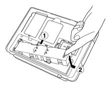
**5.** Remove the old batteries and install 6 new AA-size alkaline batteries of the same type into the main battery case carefully, observing the correct polarity as shown below.
