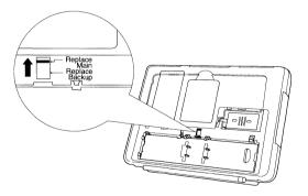
**4.** With sliding the main battery lock to "Release" (①), remove the main battery case by hooking a finger into the groove on the top of the battery case(②).
