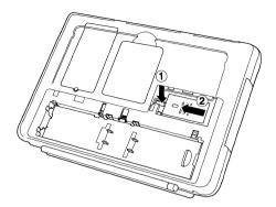
**3.** Install a lithium backup battery (CR2032) into the left slot with the – side down and one into the right slot with + side down.
