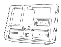
It takes about 2 hours to fully charge a battery. A fully charged battery can run the PT-9000 for about 12 hours.
