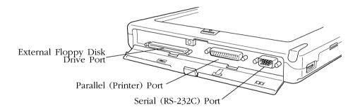
The rear panel of the unit has a compartment containing three connectors. Open the cover by pushing down the catch and swinging the cover downwards.
