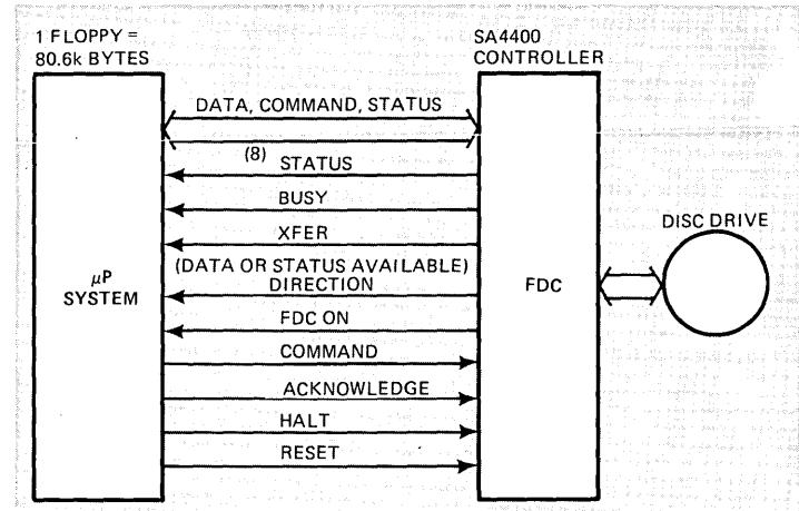
**Fig 5—A typical mini-floppy controller, the Shugart SA4400, generates ten classes of signals to interface with a μP system.**
