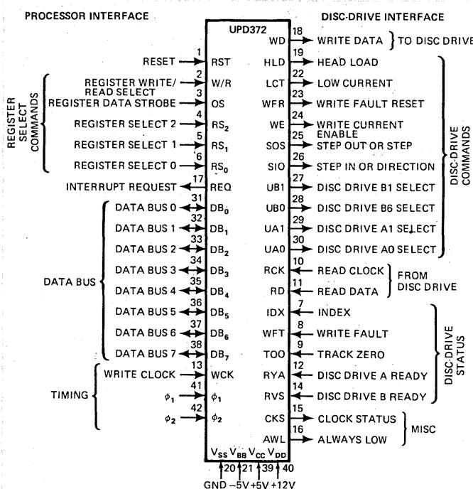
**Fig 7—Another controller chip, the NEC UPD372, can handle up to four drives simultaneously.**
