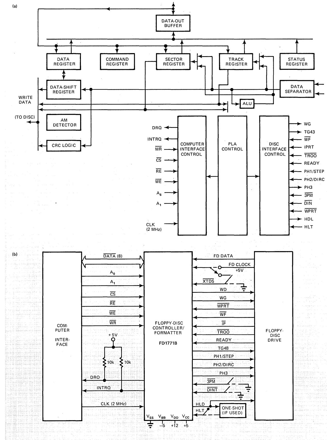
**Fig 6—Internal architecture of the Western Digital FD1771B floppy-disc controller chip (a) consists of five functional blocks, six registers and two interfaces. A complete μP-to-floppy interface utilizing this chip appears in (b).**
