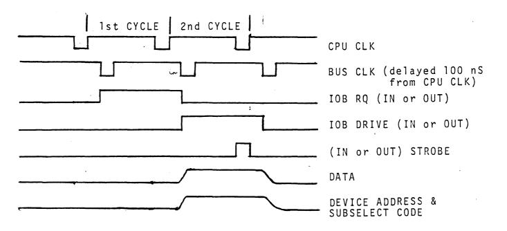
Figure 6-3 [ IOT IN & OUT TIMING ]
