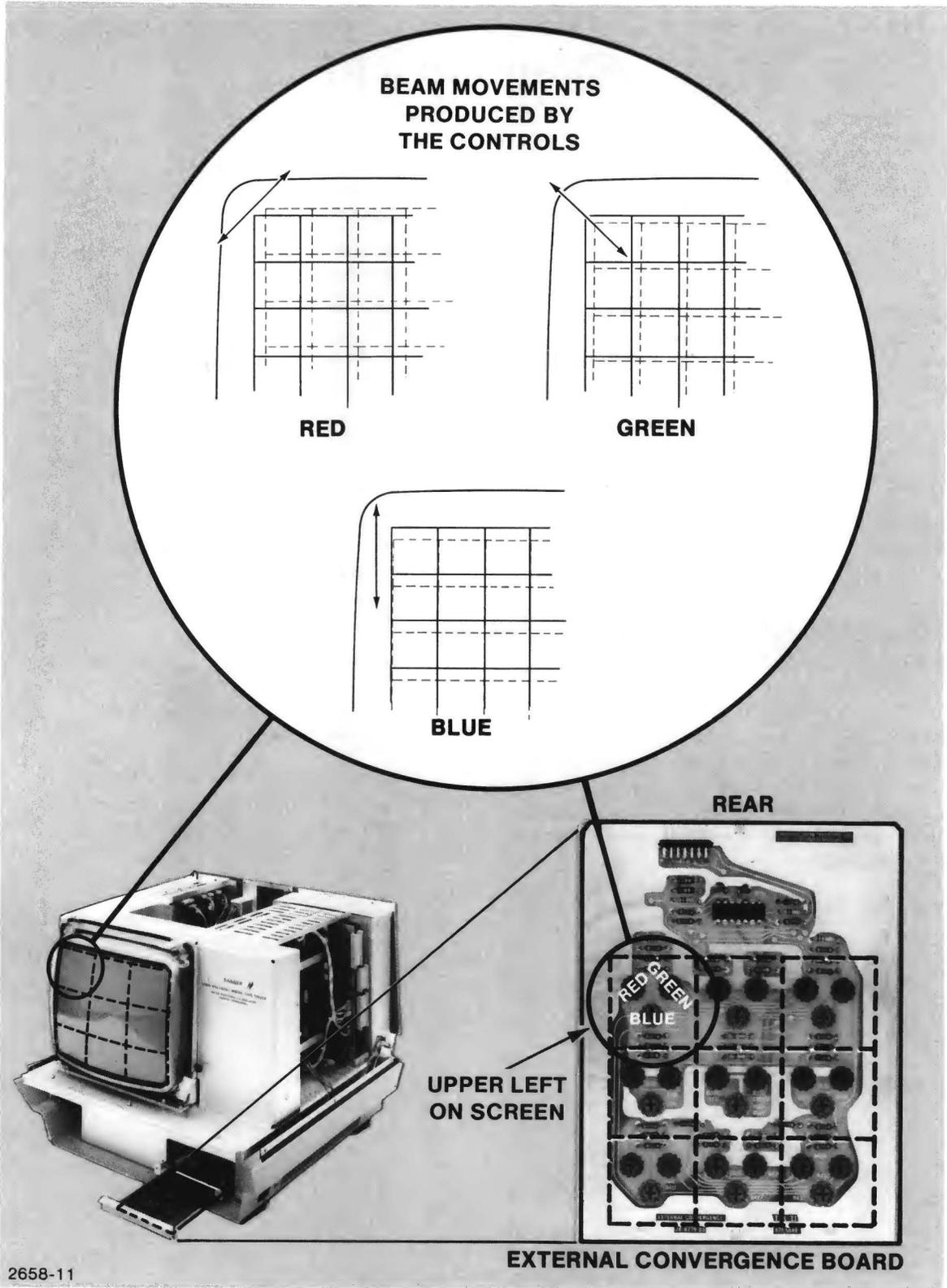
Figure I-1. Adjusting the External Convergence Board.
