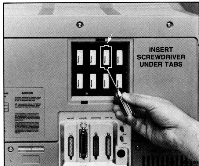
Figure B-2. Replacing the ROMs.
