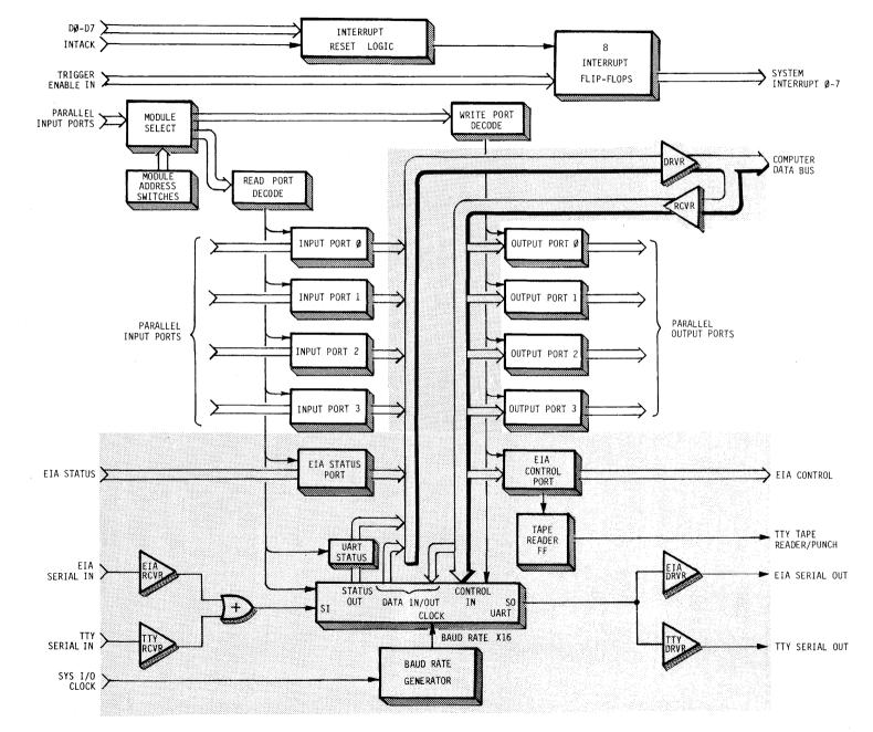
FIGURE 7-2 SERIAL I/O PORTS
