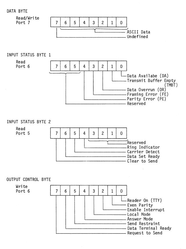
FIGURE 7-3 SERIAL PORT BYTE FORMATS
