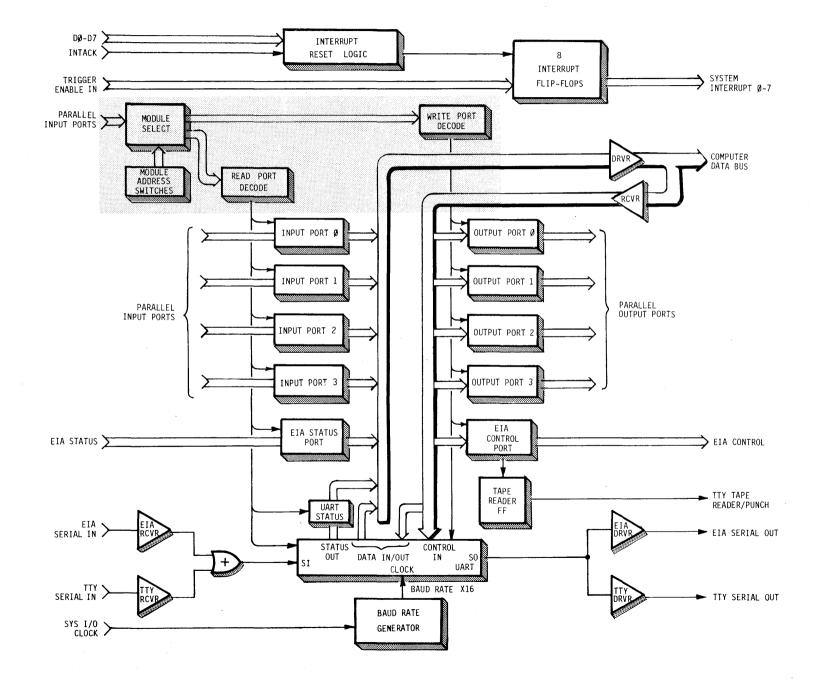
FIGURE 7-4 MODULE AND PORT ADDRESS CONTROL
