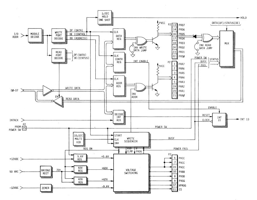
the module selected signal is further decoded to recognize a read to DE or DF. This enables the data drivers onto the system bus. Address bit 0, signifying a DE or DF command controls the MUX, routing PROM data or write status to the drivers.
