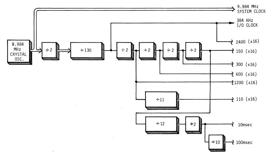
FIGURE 3-12 BAUD RATE AND TIMER LOGIC
