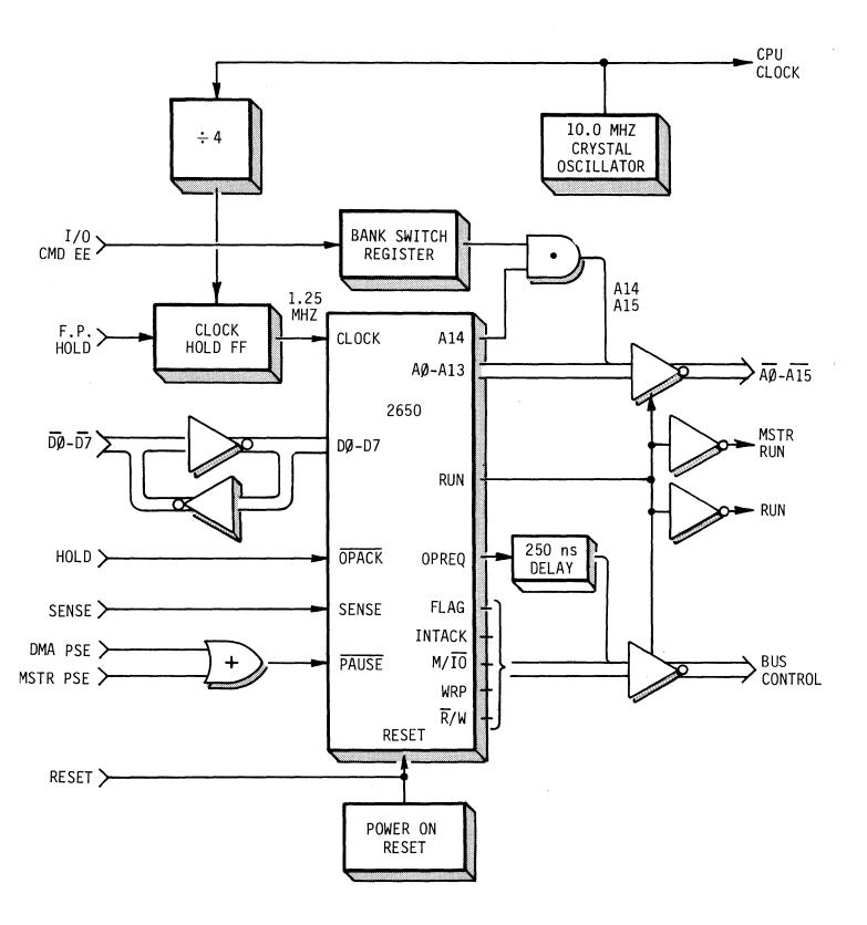
FIGURE 3-2 2650 PROCESSOR AND SUPPORT
