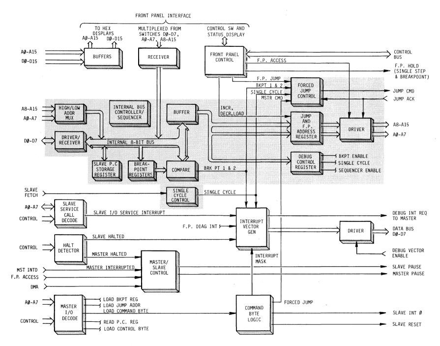
FIGURE 4-3 DEBUG LOGIC
