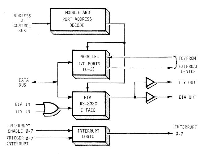
FIGURE 7-1 GP I/O SIMPLIFIED BLOCK DIAGRAM
