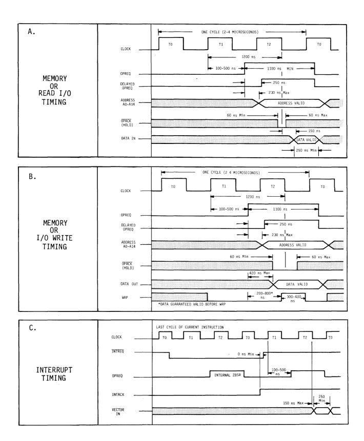
FIGURE 3-4 MASTER CPU TIMING
