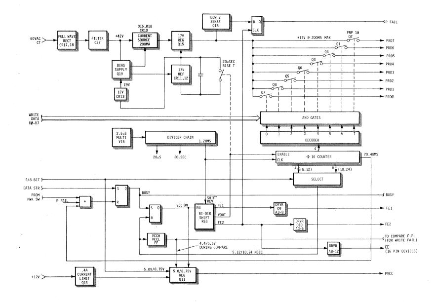
FIGURE 8-8 82S115 PROM PROGRAMMER WRITE WAVEFORM GENERATOR
