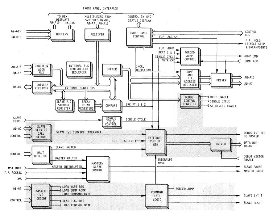
FIGURE 4-4 I/O COMMANDS AND INTERRUPTS
