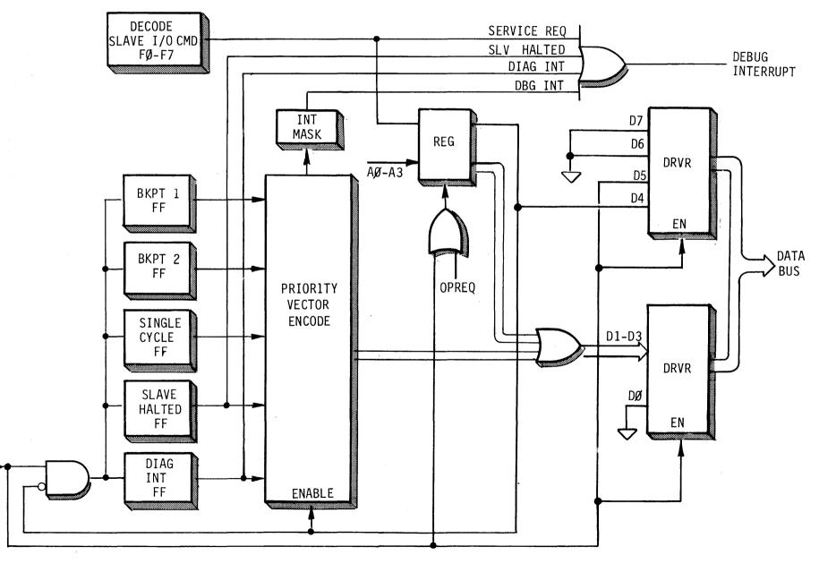
FIGURE 4-9 DEBUG INTERRUPT LOGIC
