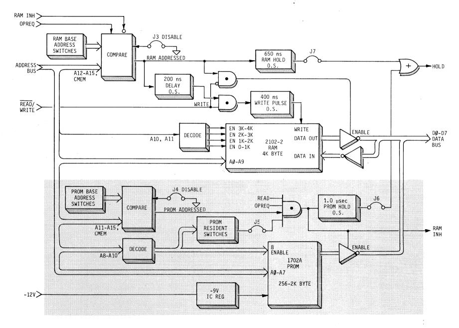
FIGURE 5-1 RAM/PROM MODULE BLOCK DIAGRAM
