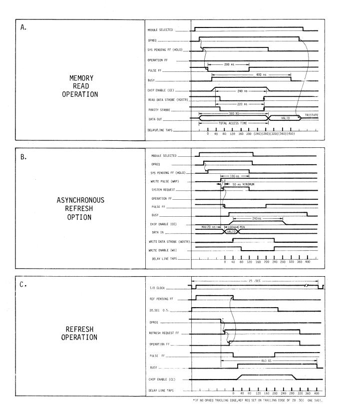
FIGURE 6-13 TIMING DIAGRAMS
