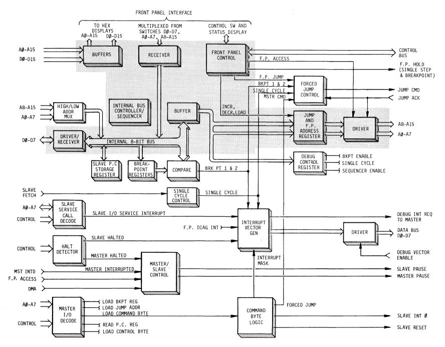
FIGURE 4-5 FRONT PANEL INTERFACE
