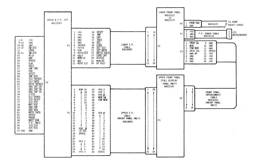
FIGURE 4-13 DEBUG AND FRONT PANEL INTERCONNECT
