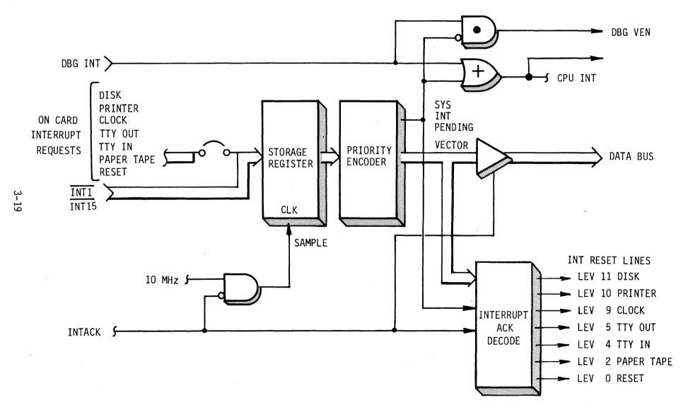
FIGURE 3-10 MASTER CPU INTERRUPT LOGIC
