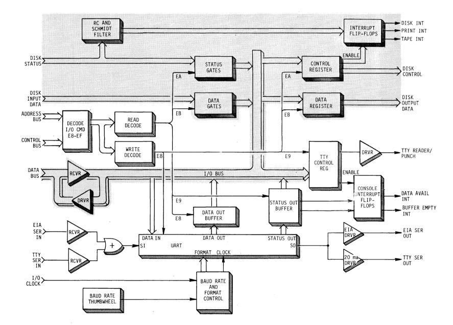
FIGURE 3-7 MASTER CPU DISK I/O BLOCK DIAGRAM
