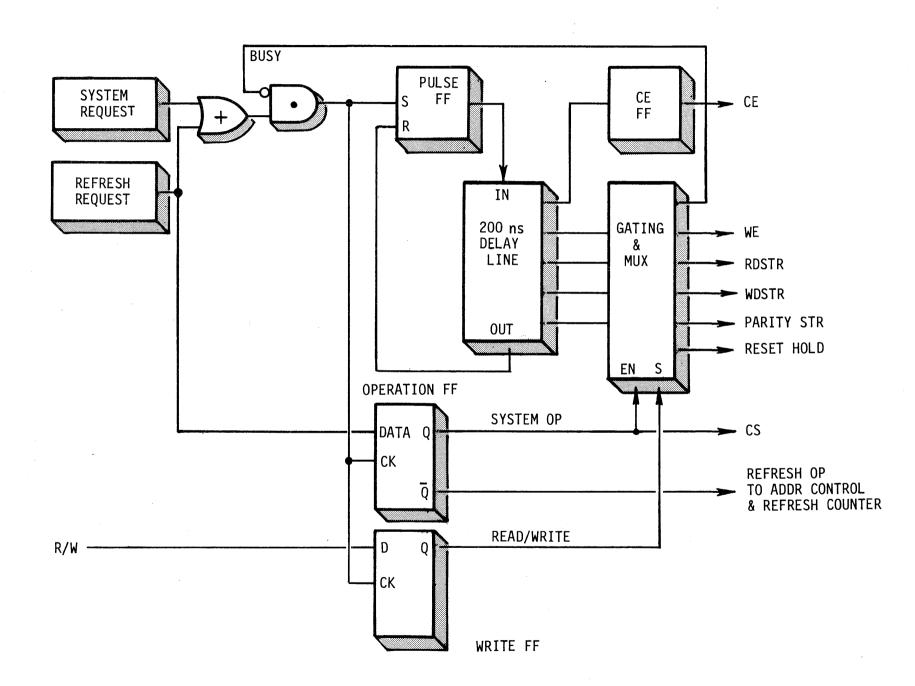
FIGURE 6-12 OPERATION CONTROL AND TIMING BLOCK DIAGRAM
