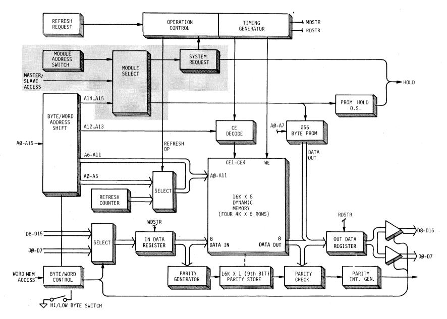
FIGURE 6-4 MODULE SELECT AND SYSTEM REQUEST LOGIC
