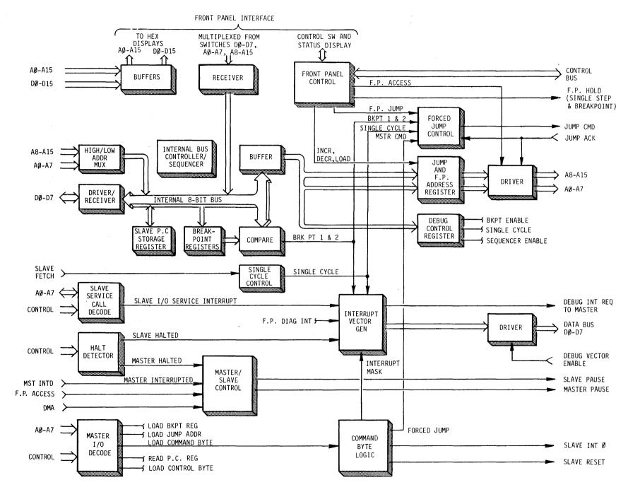
FIGURE 4-1 DEBUG AND FRONT PANEL I/O BLOCK DIAGRAM
