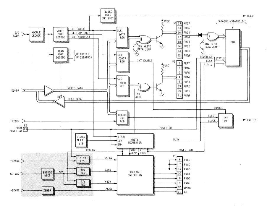
FIGURE 8-4 1702A PROM PROGRAMMER BLOCK DIAGRAM
