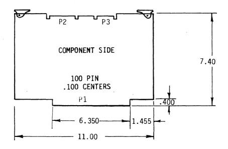
FIGURE 3-13 MASTER CPU ENVIRONMENTAL, POWER AND PHYSICAL REQUIREMENTS
