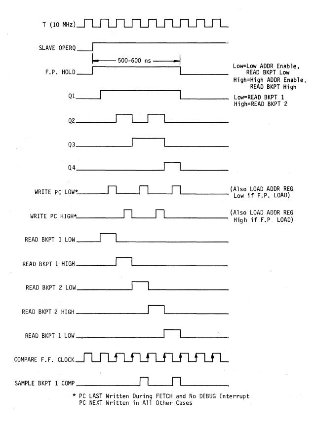
FIGURE 4-11 SEQUENCER TIMING
