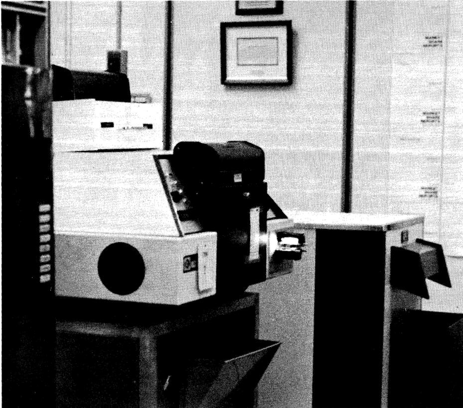
Fig. 4. Once translated by the Kennedy, the typesetting specifications and text data are sent to the Photon typesetting processor.
