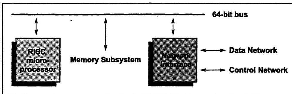
Figure 2. The components of a typical processing node.
