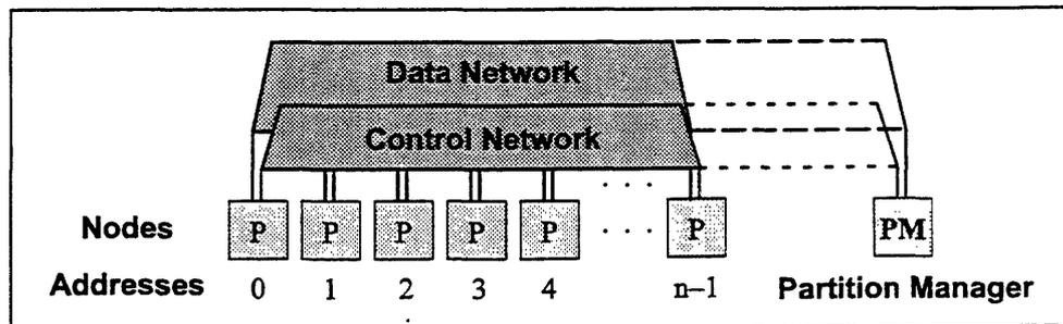
Figure 6. Addressing of nodes in a partition.
