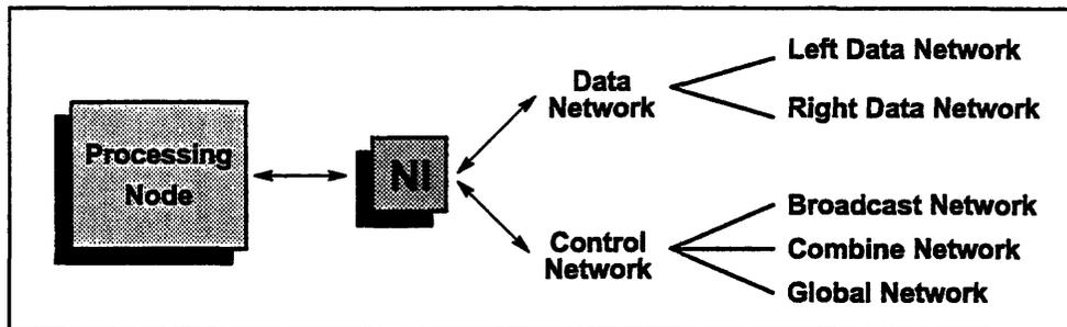
Figure 4. The NI provides access to the facilities of the Data and Control Networks.
