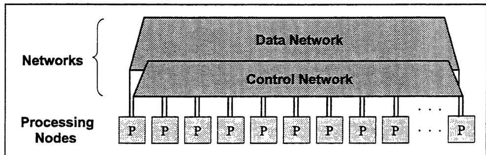
Figure 1. The CM-5 system: Processing nodes linked by Data and Control Networks.
