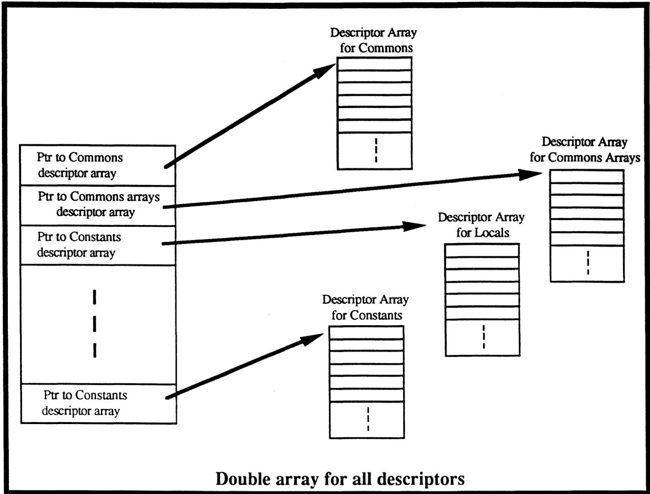
One significant advantage of this data structure is how **call** becomes simplified with respect to handling local variables. To give the program a new set of local variables, all that has to happen is save the address of the caller's local variables descriptor table and make the corresponding entry in the first array point to a newly allocated callee local variables descriptor table.
