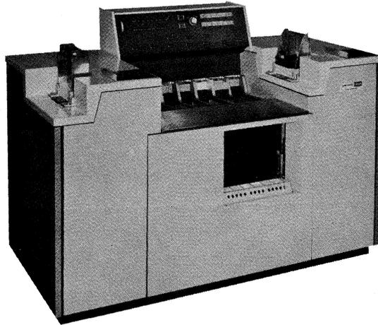
Figure 4-4. UNIVAC 1001 Card Controller
