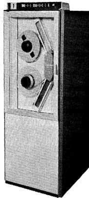
Figure 4-3. UNISERVO VI C Magnetic Tape Unit
