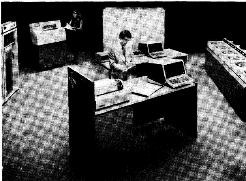
*The 1100/60 System supports up to 4 central processors and up to 8192K words of main memory. A single processor configuration can include a maximum of four consoles; a multiprocessor configuration, a maximum of seven consoles.*
