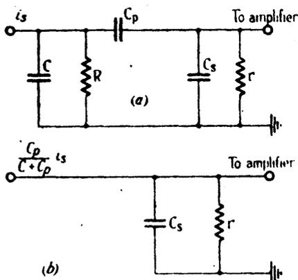
Fig. 4.—Amplifier input circuit.
