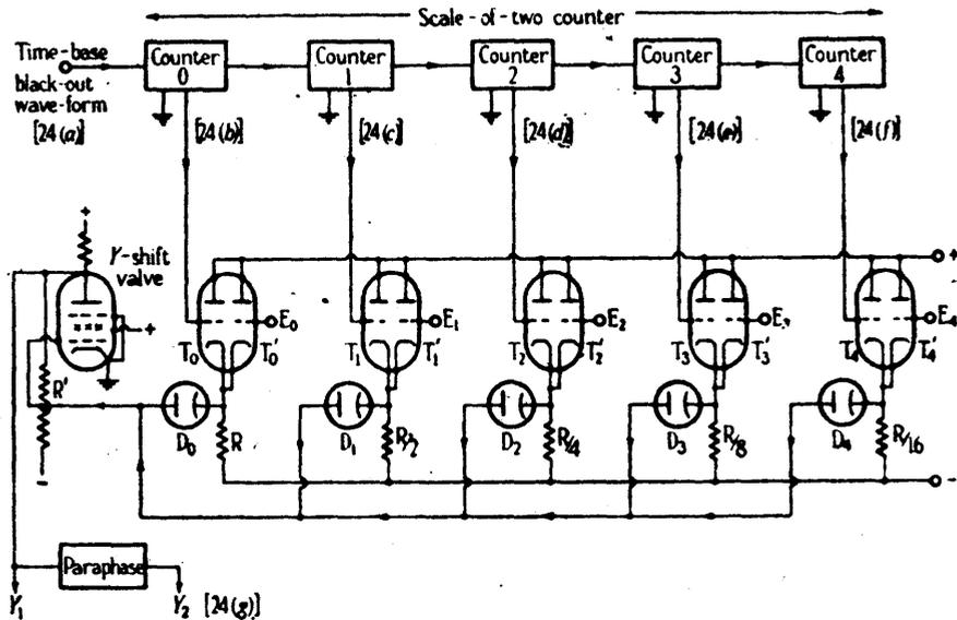
Fig. 23.—Simple Y-shift generator.
